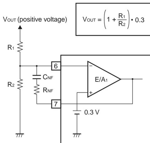
(2) When setting a positive output voltage using error amplifier E/A<sub>2</sub>.
