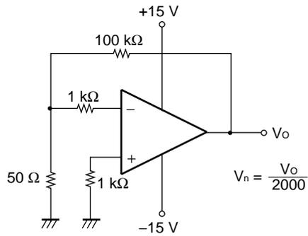
Figure2 Channel Separation Measurement Circuit
