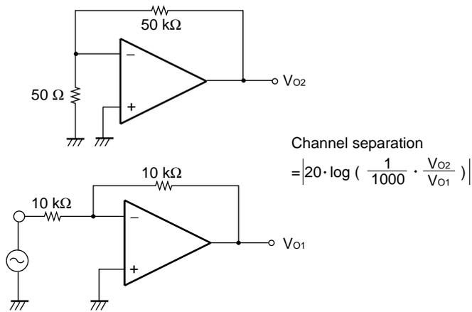
TYPICAL PERFORMANCE CHARACTERISTICS ( $T_A = 25^\circ\text{C}$ , TYP.)
