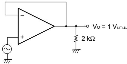
Fig. 2 Noise Measurement Circuit (RIAA)
