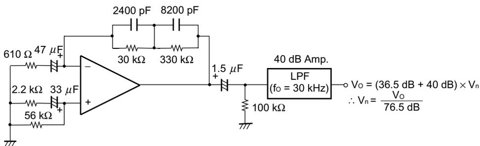
Fig. 3 Flat Noise Measurement Circuit (FLAT + JIS A)
