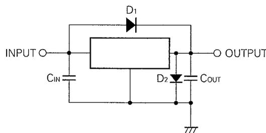
C<sub>IN</sub>: Required if regulator is located an appreciable distance from power supply filter (More than 2.2 μF)
