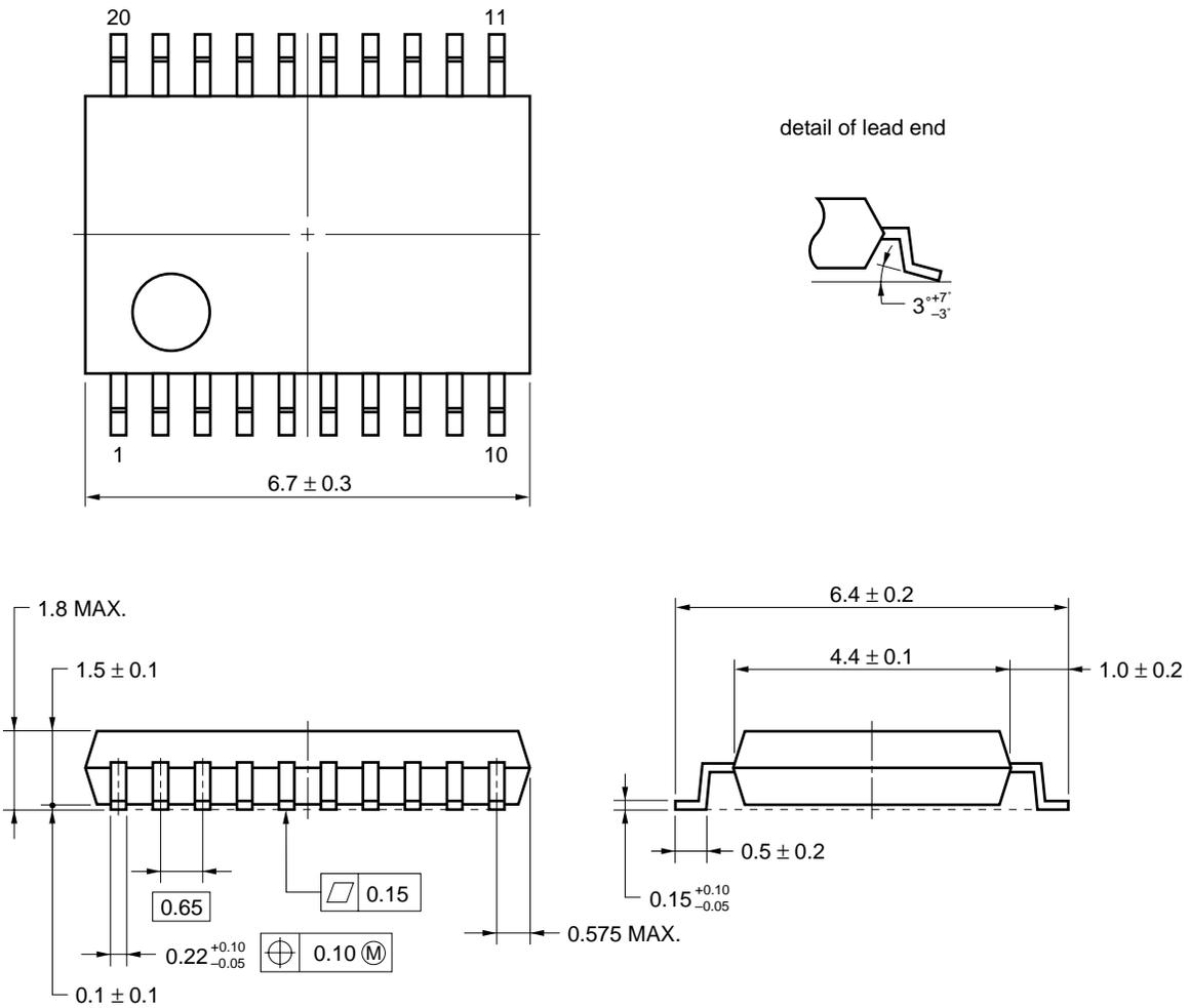
**NOTE** Each lead centerline is located within 0.10 mm of its true position (T.P.) at maximum material condition.
