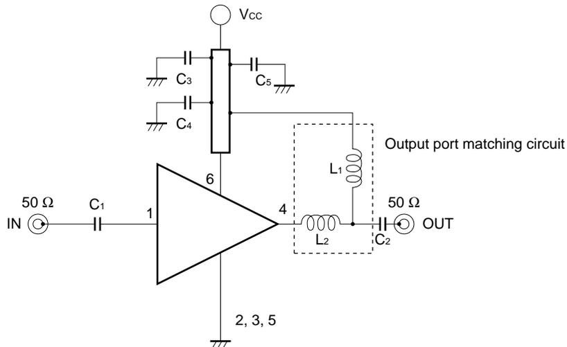
ILLUSTRATION OF THE TEST CIRCUIT ASSEMBLED ON EVALUATION BOARD
