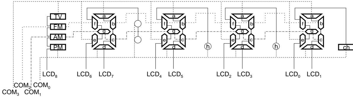
Relationship between the segment and common pins and the display segments on the LCD panel
