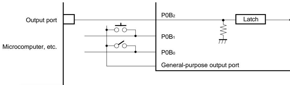
Halt can be released by another microcomputer, etc. as shown in the figure above.
