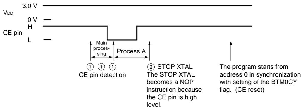
**14.4 DEVICE OPERATION IN THE HALT AND CLOCK-STOP STATES**
