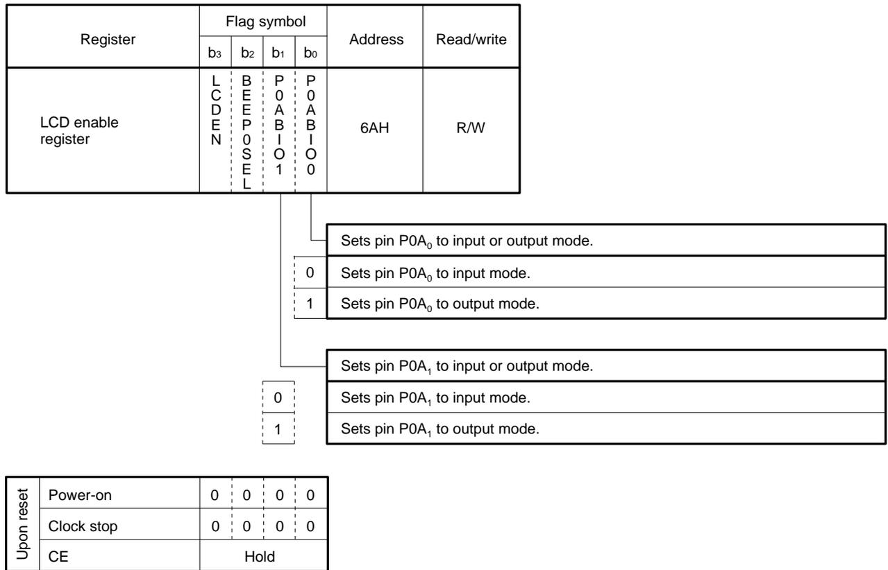
**9.2.4 Using an I/O Port as an Input Port**
