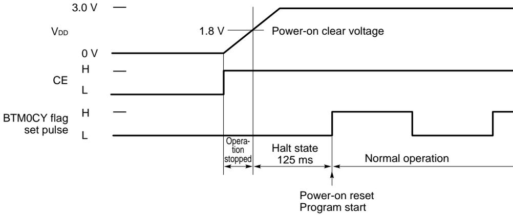
(b) When CE Pin Raised in Halt State
