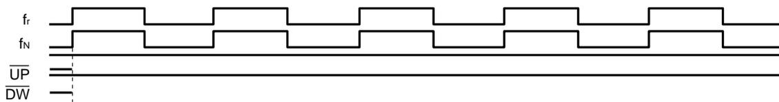
**(d) When  $f_N$  frequency lower than  $f_r$  frequency**
