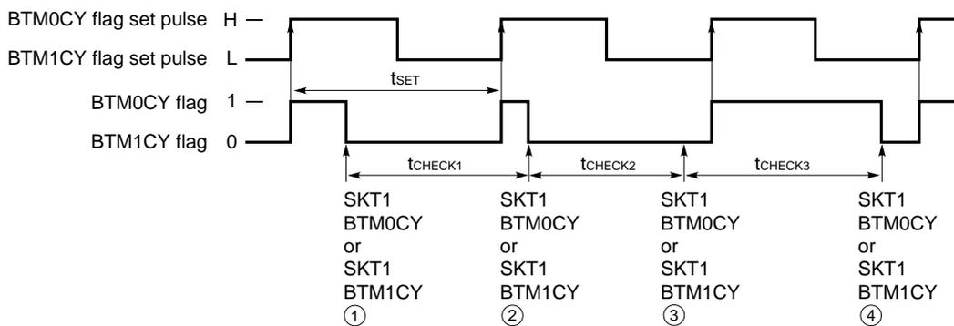
As shown in Fig. 10-4, when the BTM0CY and BTM1CY flags are detected at ②, the timer is updated because the flag is "1". When the flag is detected at ③, because it is "0", the timer is not updated until it is detected again at ④. Therefore, the timer is incremented by t<sub>CHECK3</sub>.
