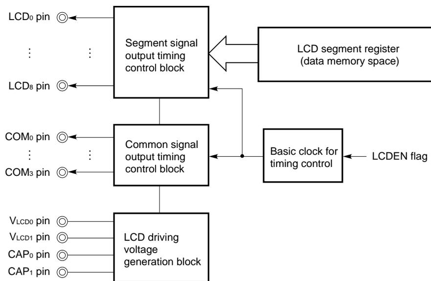
**Remark** LCDEN (bit 3 of the LCD enable register; see Fig. 13-6) turns the entire LCD display on or off.
