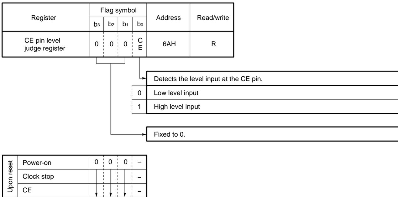
The CE flag also does not change when the CE pin receives signals having a low or high level width of less than 140 μs.
