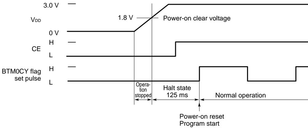
(c) When CE Pin Raised After Power-On Reset
