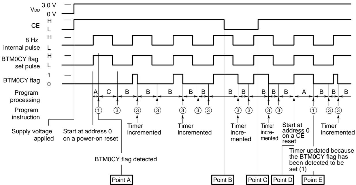
As shown in Fig. 10-6, when supply voltage VDD is applied, the 8 Hz internal pulse rises to make the program start at address 0000H.
