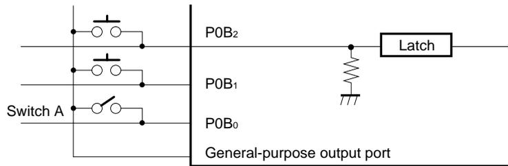
Execute a "HALT 0001B" instruction after the key source signal general-purpose output port is made high level. Note that if an alternate switch like switch A in the figure above is used, while switch A is closed, high level is applied to the P0B<sub>0</sub> pin and the halt state is immediately released.
