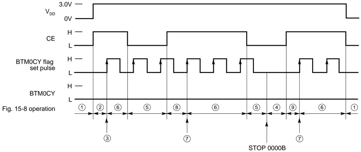
(b) When power failure detected with BTM0CY flag
