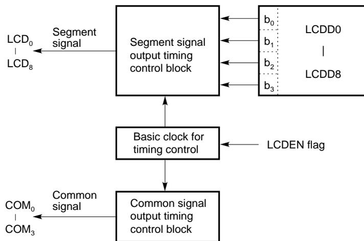
**Fig. 13-6 Configuration and Functions of LCD Enable Register**
