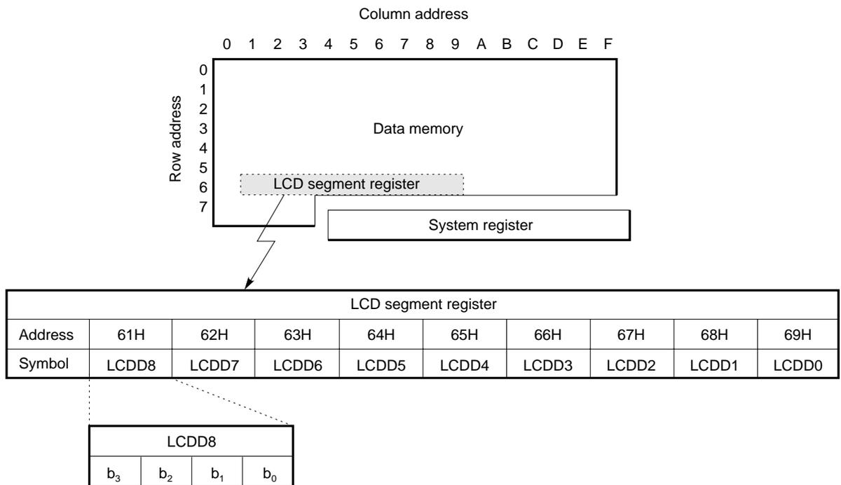
Fig. 13-4 Relationship Between LCD Segment Register and LCD Segments, and Examples of Display
