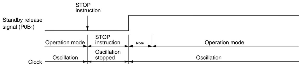
**Note** The HALT mode remains effective in this period, waiting for the generation of clock pulses to settle. An operation starts after eight clock pulses on the OSC<sub>0</sub> pin are counted.
