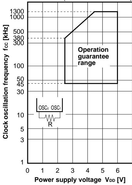
**R<sub>osc</sub> vs. V<sub>DD</sub> for Operation Guarantee Range**
