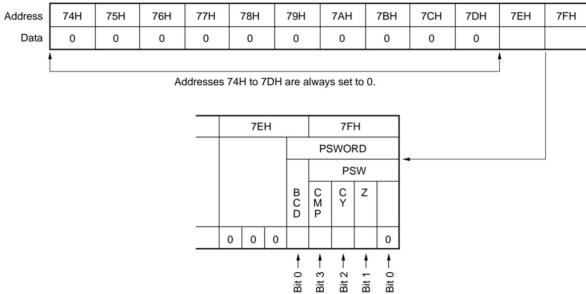
Bit 0 at address 7EH and all four bits at address 7FH (PSW) are assigned to the program status word.
