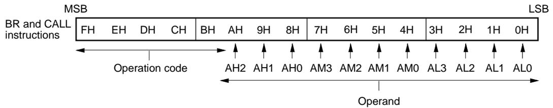
When the assembler is not used and a BR or CALL instruction is used, AH2 and AH1 must be set to 0. Reset input clears all bits of the program counter to 0.
