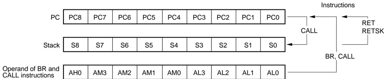
In Fig. 2-1, AHn, AMn, and ALn (0 ≤ n ≤ 3) indicate bit positions in a 16-bit instruction as follows:
