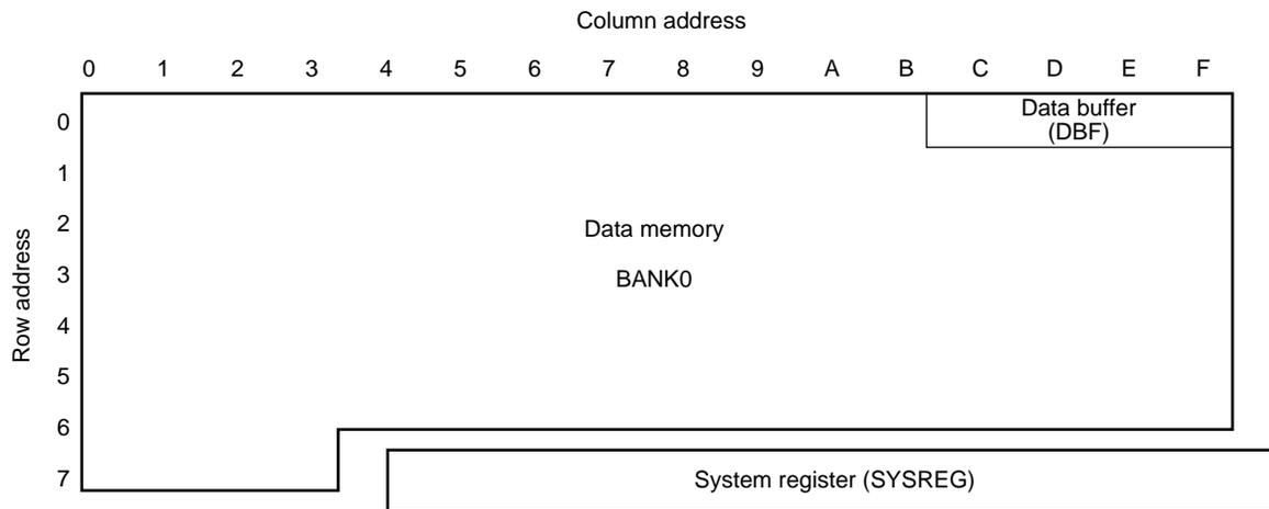
Figure 9-2 shows the configuration of the data buffer. As shown in this figure, the data buffer consists of 16 bits of the data memory, with the bit 0 of address 0FH as the LSB and bit 3 of address 0CH as the MSB.
