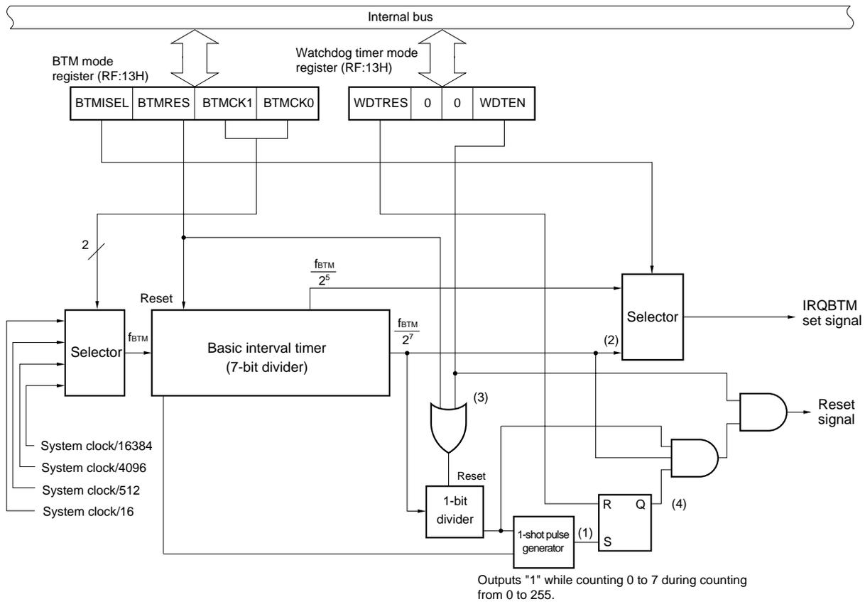
**Remark** (1) to (4) in the figure correspond to the signals in the timing chart in Figure 13-4.
