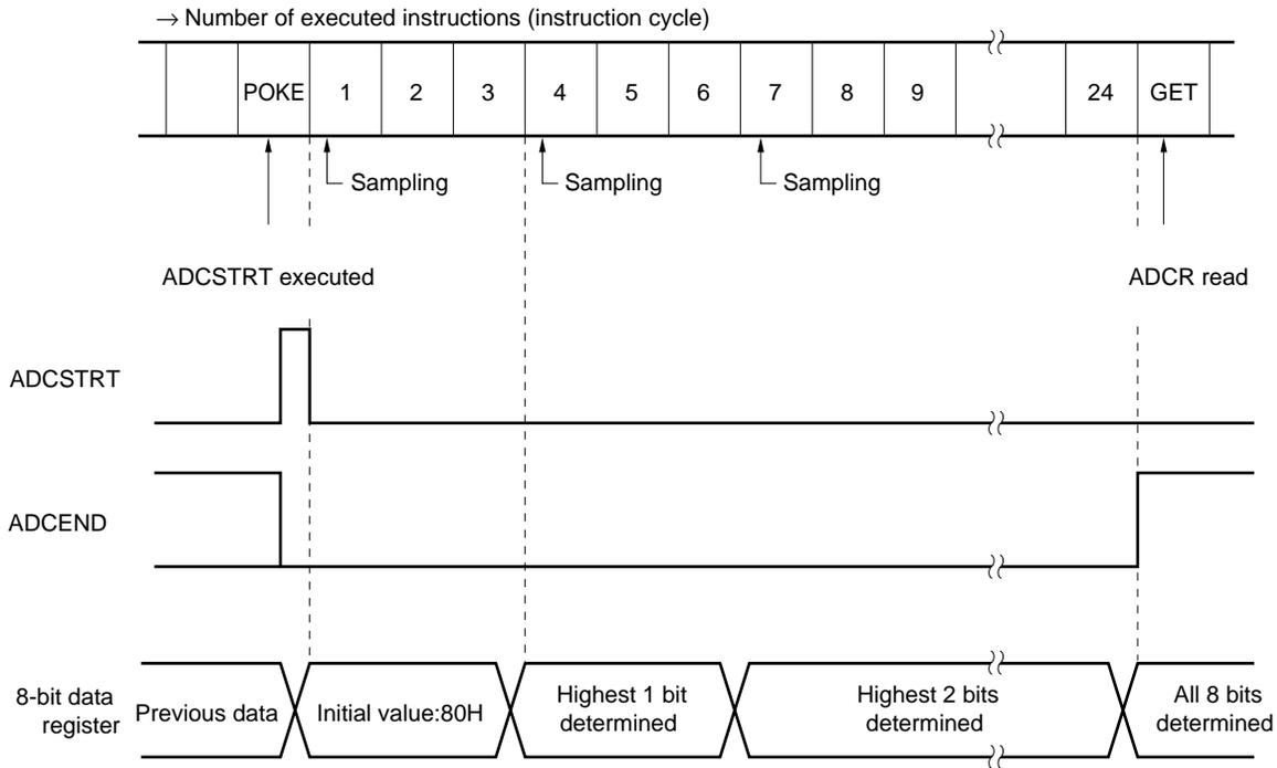
**Caution** Sampling is performed eight times while A/D conversion is executed once. If the analog input voltage changes heavily during A/D conversion, A/D conversion cannot be performed accurately. To obtain an accurate conversion result, it is necessary to minimize the changes in the analog input voltage during A/D conversion.
