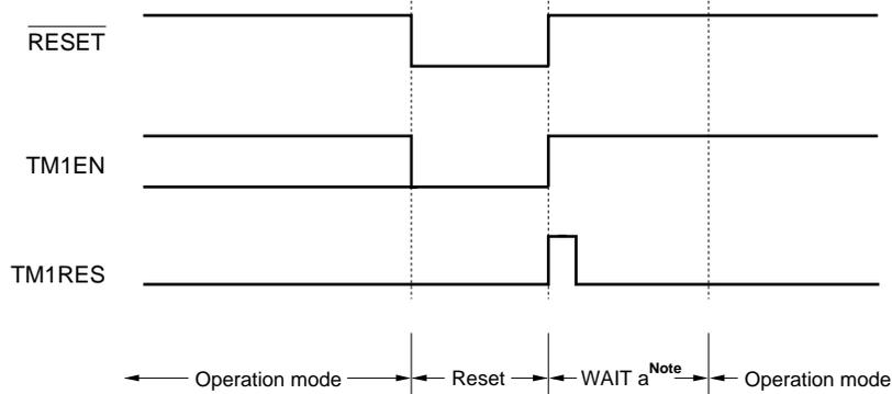
**Note** Oscillation stabilization wait time. An operation mode is set when system clock is counted  $128 \times 256$  times by timer 1 (time required to executed 2048 instructions: approx. 4 ms at 8 MHz).
