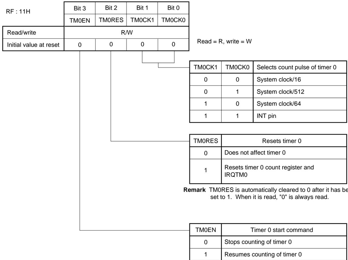
**Remark** TM0RES is automatically cleared to 0 after it has been set to 1. When it is read, "0" is always read.
