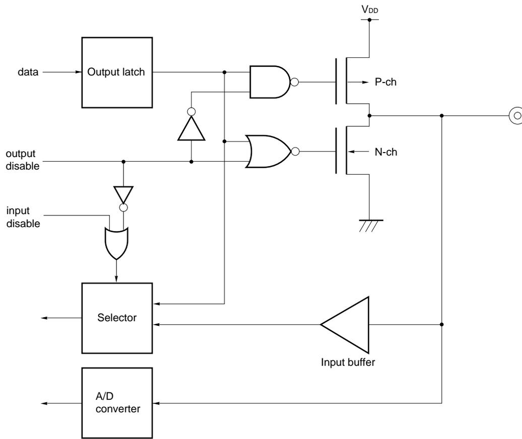
(3) P0D<sub>3</sub>/TM1OUT and P0D<sub>1</sub>/SO
