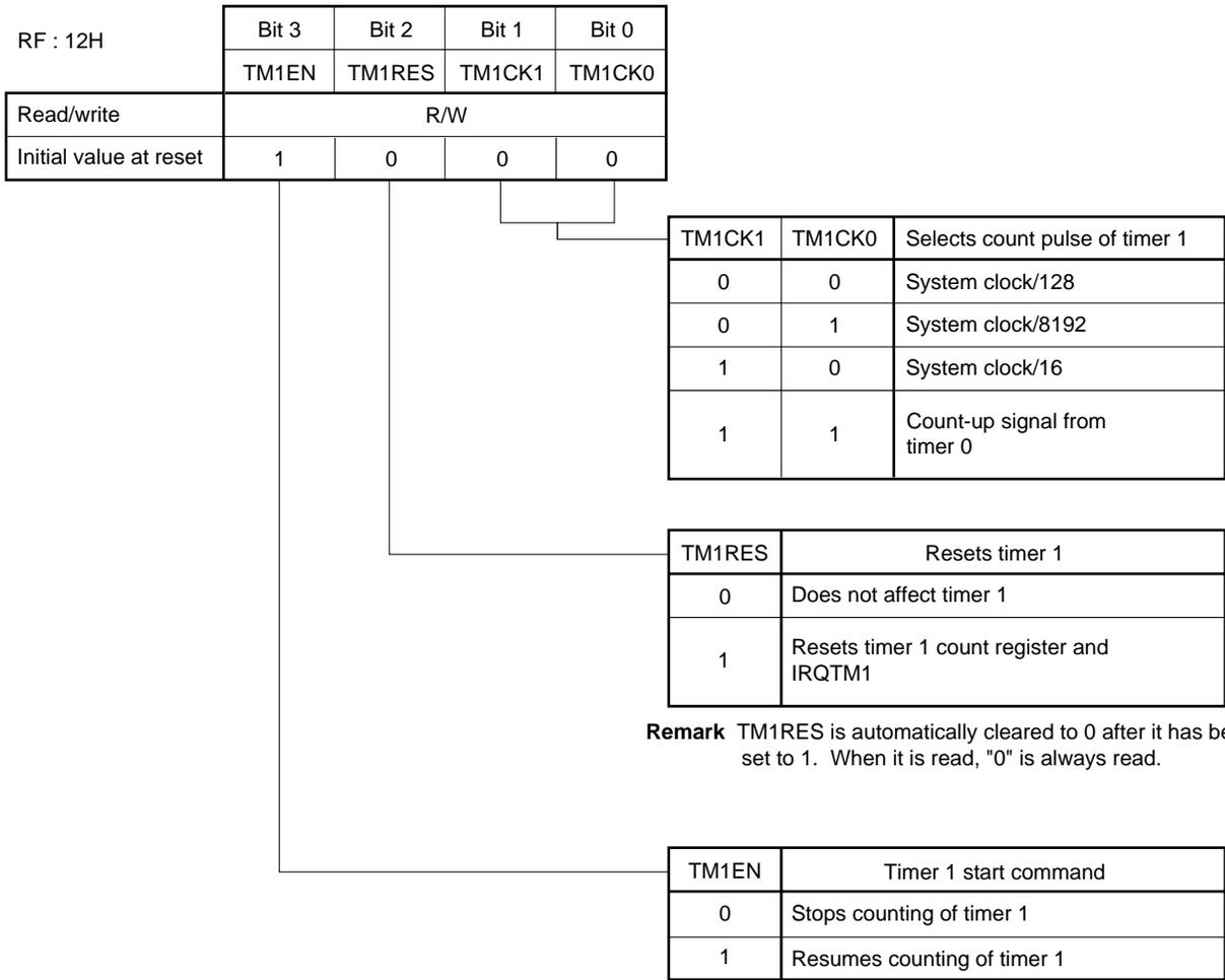
**Remark** TM1RES is automatically cleared to 0 after it has been set to 1. When it is read, "0" is always read.
