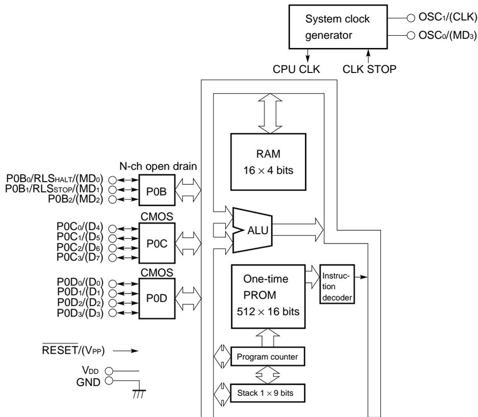
**Remark** Pin names enclosed in parentheses are used in PROM programming mode.
