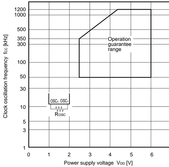
**$R_{osc}$  vs.  $V_{DD}$  for Operation Guarantee Range ( $T_A = -40$  to  $+85$  °C)**
