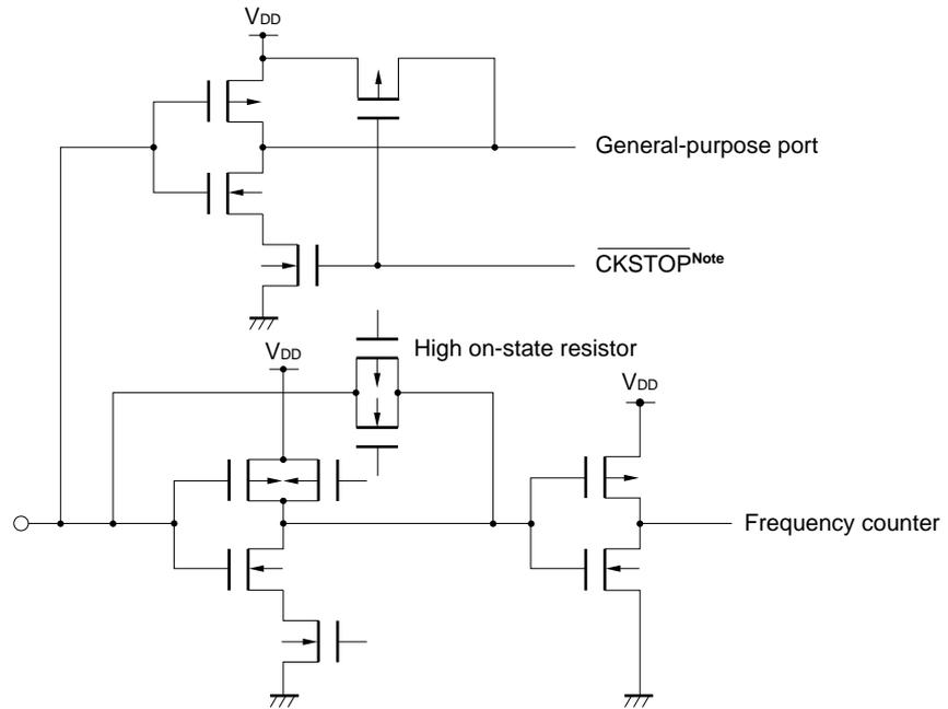
**Note** In this circuit, a current drained by noise does not increase even if the circuit is in the floating state, because of the internal signal being output when the clock stop instruction is executed.
