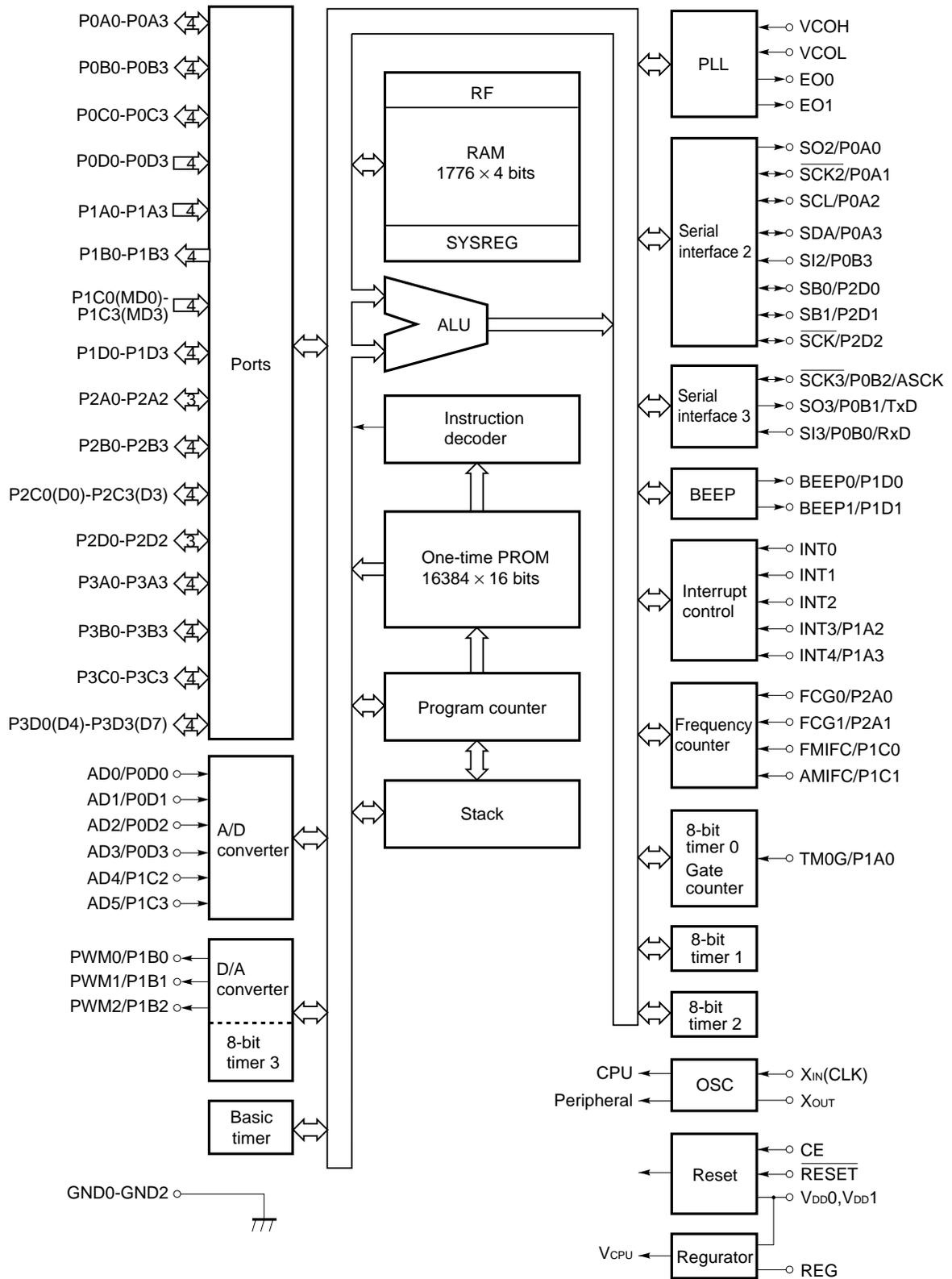
**Remark** Pins enclosed in parentheses are used in PROM programming mode.
