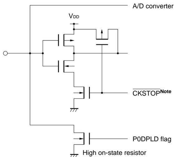
**Note** In this circuit, a current drained by noise does not increase even if the circuit is in the floating state, because of the internal signal being output when the clock stop instruction is executed.
