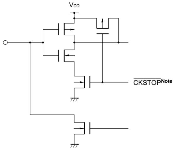
**Note** In this circuit, a current drained by noise does not increase even if the circuit is in the floating state, because of the internal signal being output when the clock stop instruction is executed.
