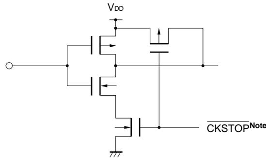
**Note** In this circuit, a current drained by noise does not increase even if the circuit is in the floating state, because of the internal signal being output when the clock stop instruction is executed.
