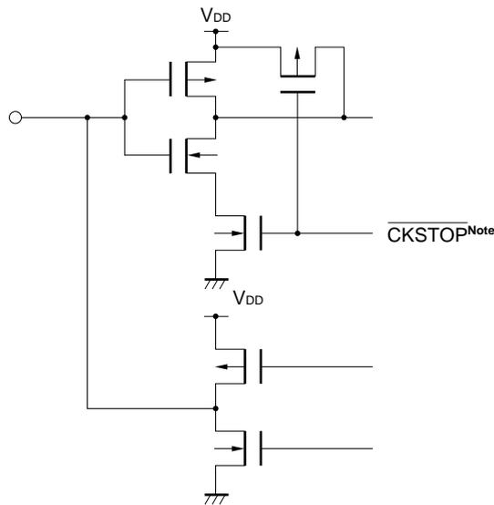
**Note** In this circuit, a current drained by noise does not increase even if the circuit is in the floating state, because of the internal signal being output when the clock stop instruction is executed.
