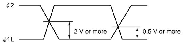
**Remark** Adjust cross points (φ1, φ2) and (φ1L, φ2) with input resistance of each pin.
