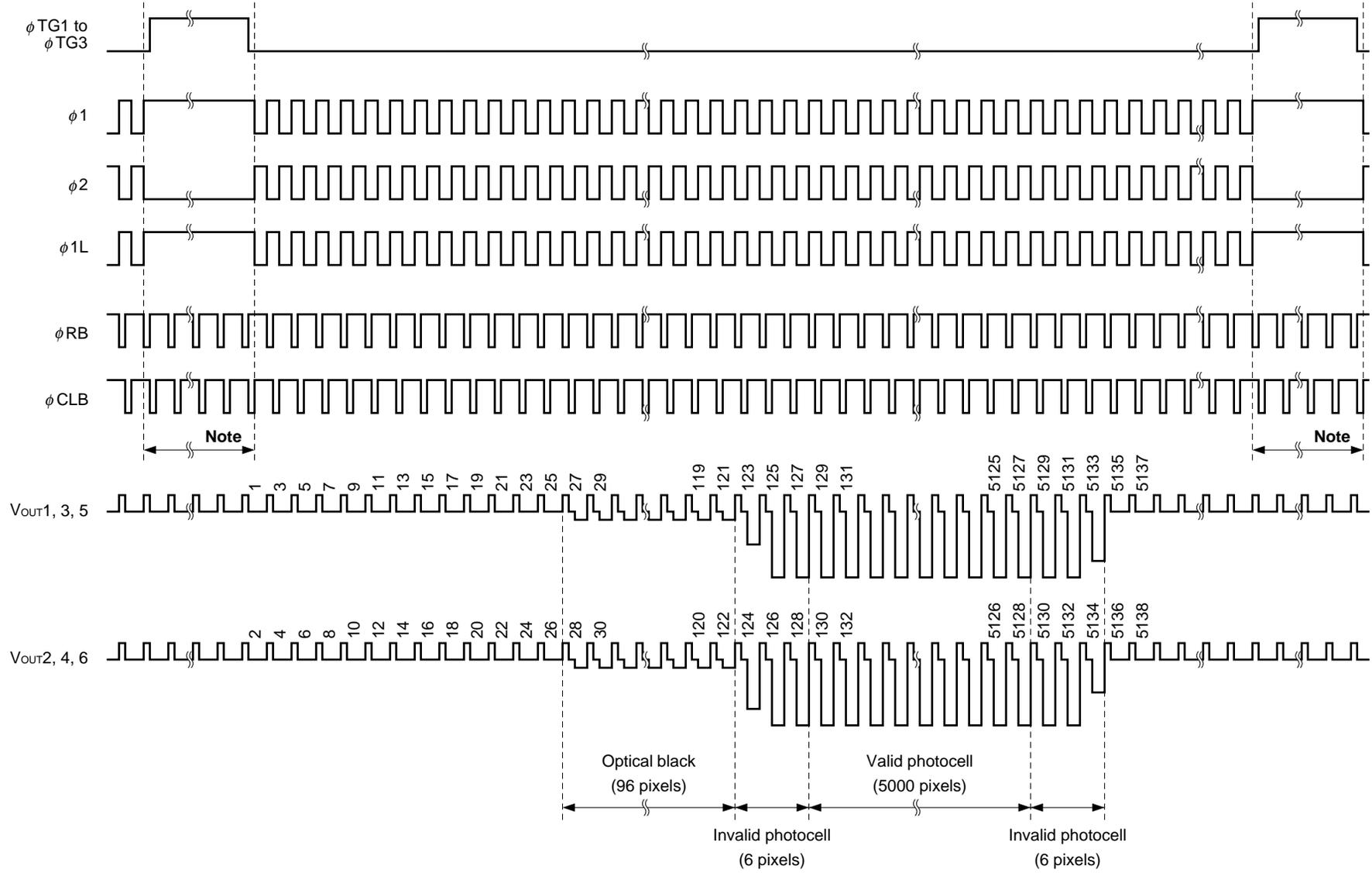
**Note** Input the  $\phi$ RB and  $\phi$ CLB pulses continuously during this period, too.
