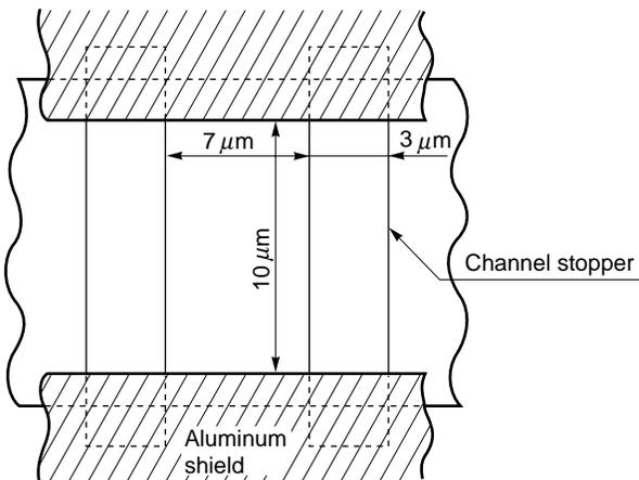
**PHOTOCELL ARRAY STRUCTURE DIAGRAM (Line spacing)**
