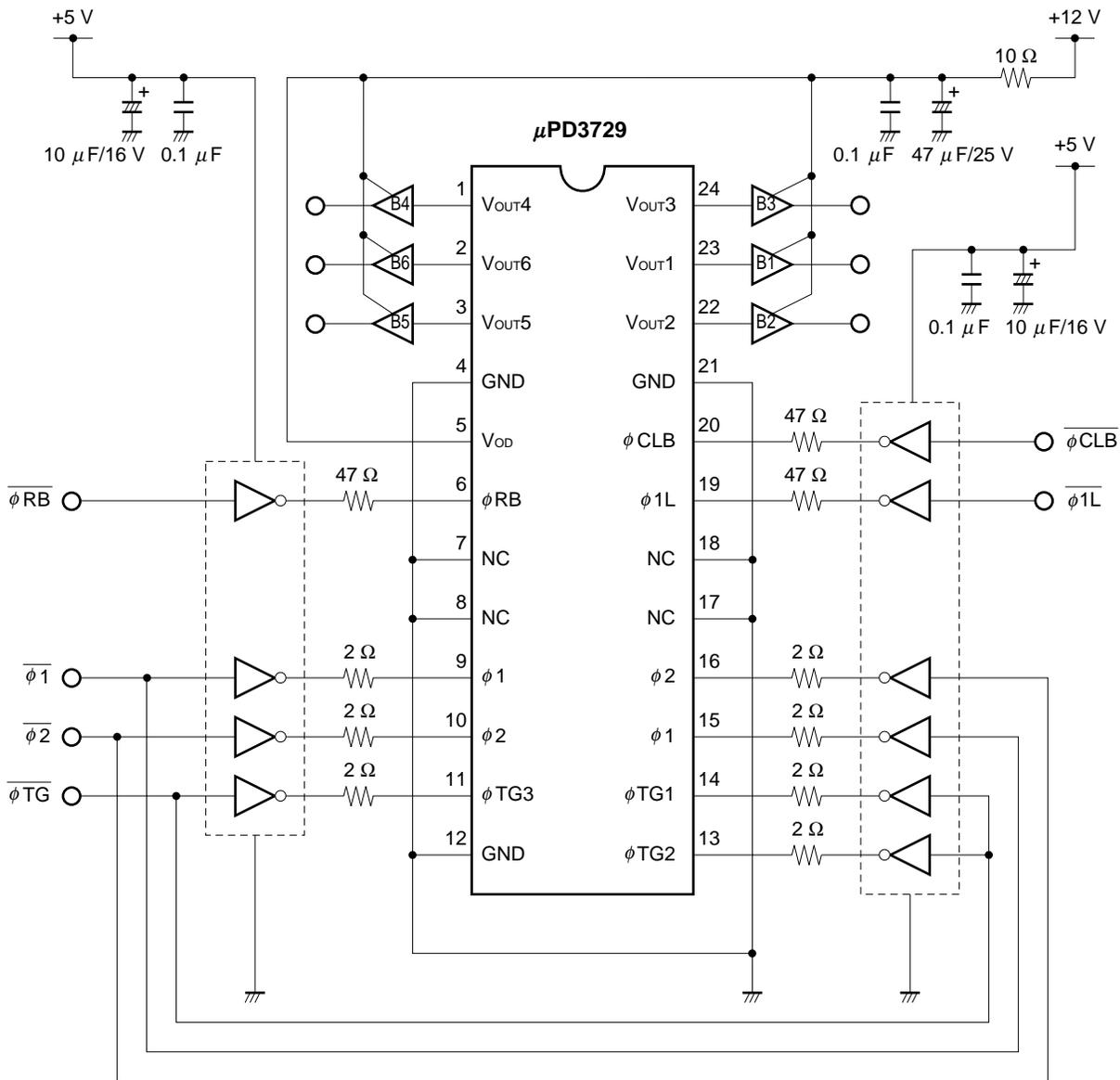
**Remark** The inverters shown in the above application circuit example are the 74AC04.
