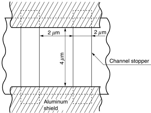
PHOTOCELL ARRAY STRUCTURE DIAGRAM
