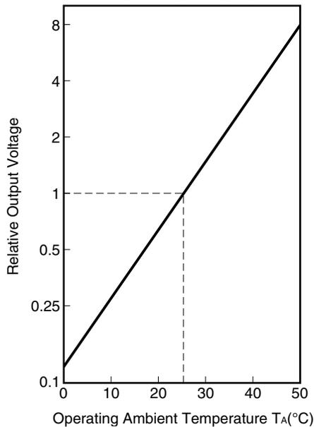
STORAGE TIME OUTPUT VOLTAGE CHARACTERISTIC ( $T_A = +25\text{ }^\circ\text{C}$ )
