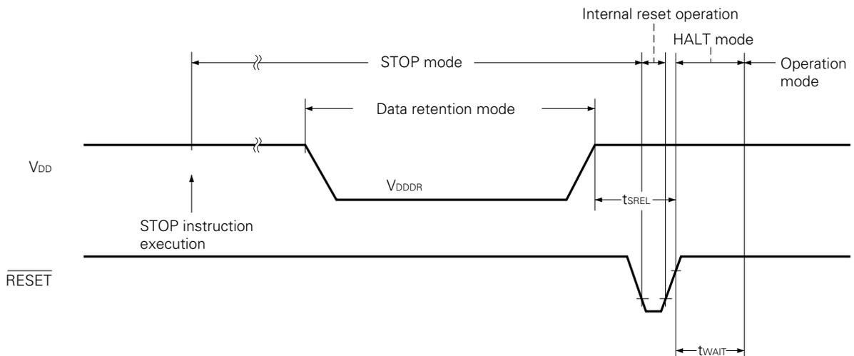
**DATA RETENTION TIMING (standby release signal: releasing STOP mode by interrupt)**
