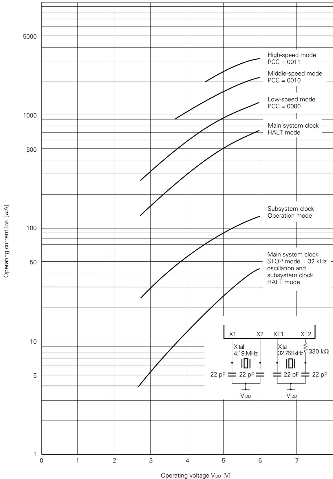
I<sub>DD</sub> vs V<sub>DD</sub> (Ceramic oscillation: 4.19 MHz)
