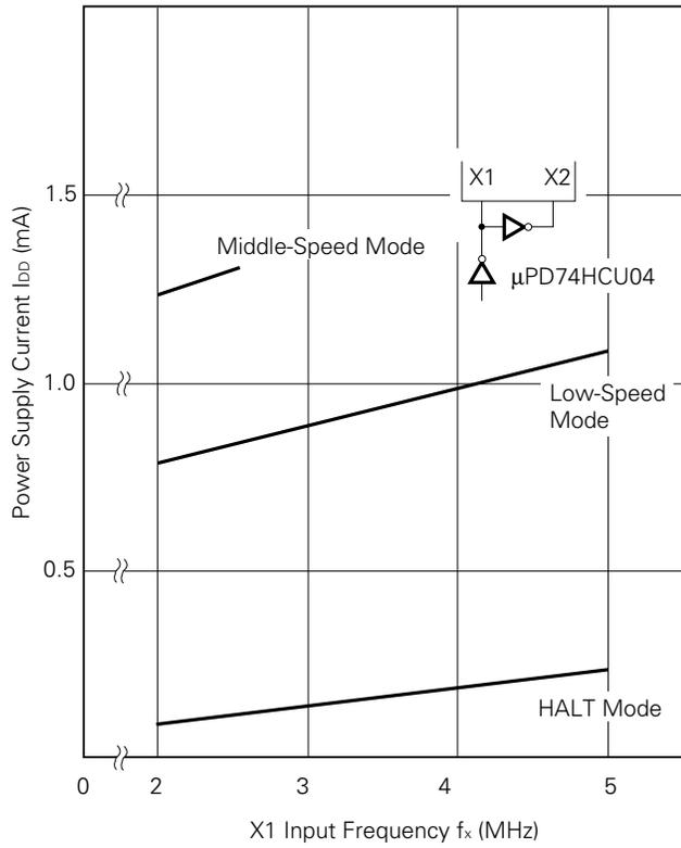
**I<sub>DD</sub> vs f<sub>x</sub> (External Clock)**
