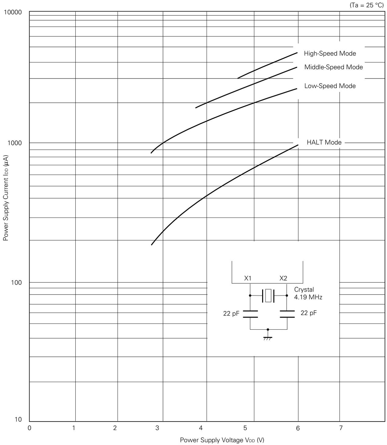
I<sub>DD</sub> vs V<sub>DD</sub> (Ceramic Oscillation)
