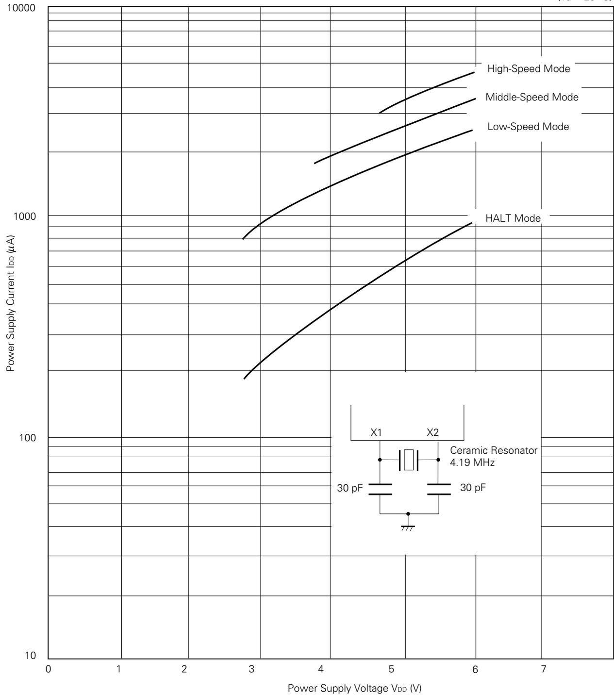
I<sub>DD</sub> vs V<sub>DD</sub> (Crystal Oscillation)
