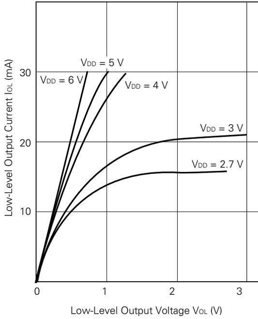
**$V_{OL}$  vs  $I_{OL}$  (Ports 0 and 2 to 9)**
