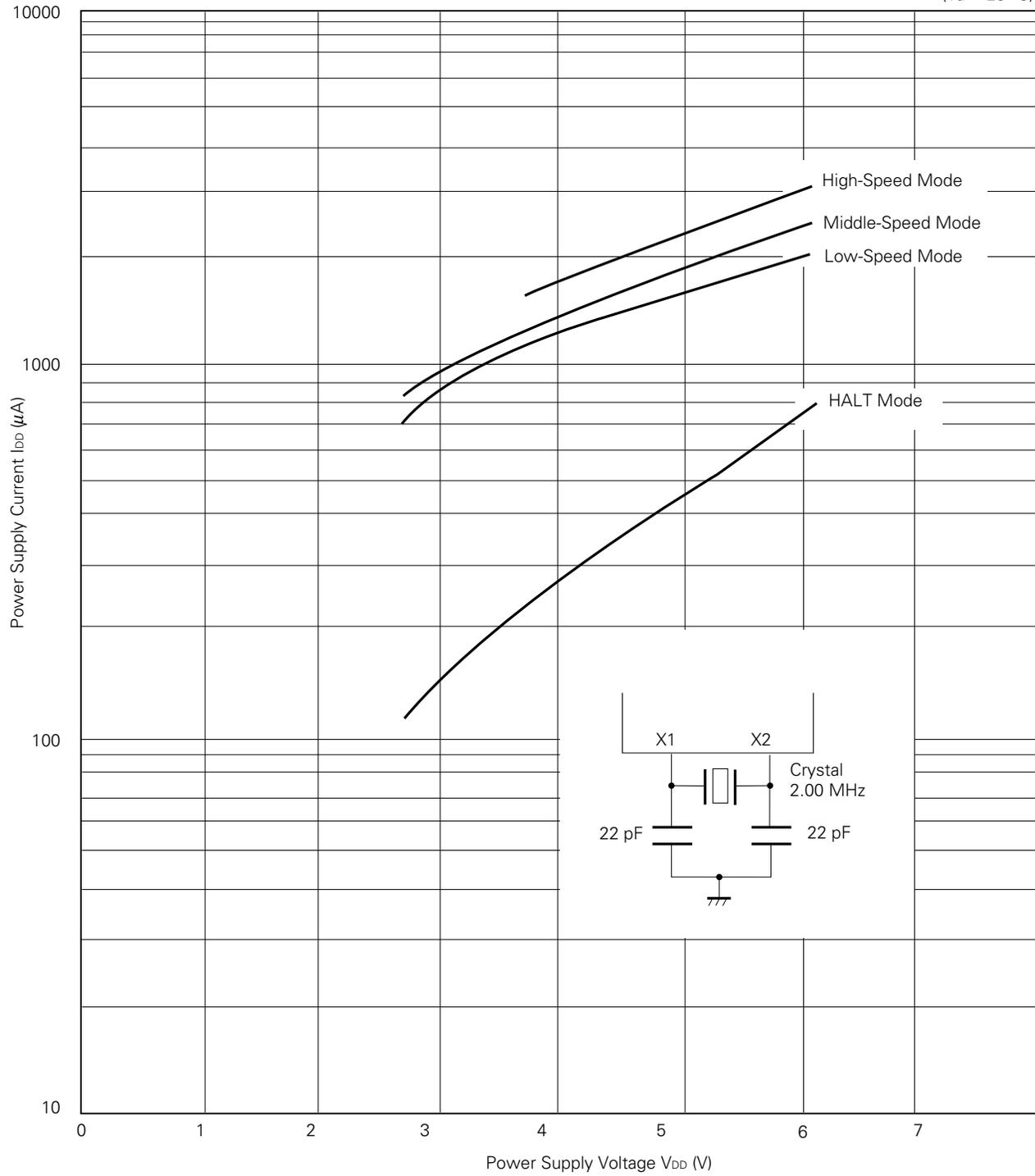
I<sub>DD</sub> vs T<sub>a</sub> (Crystal Oscillation)
