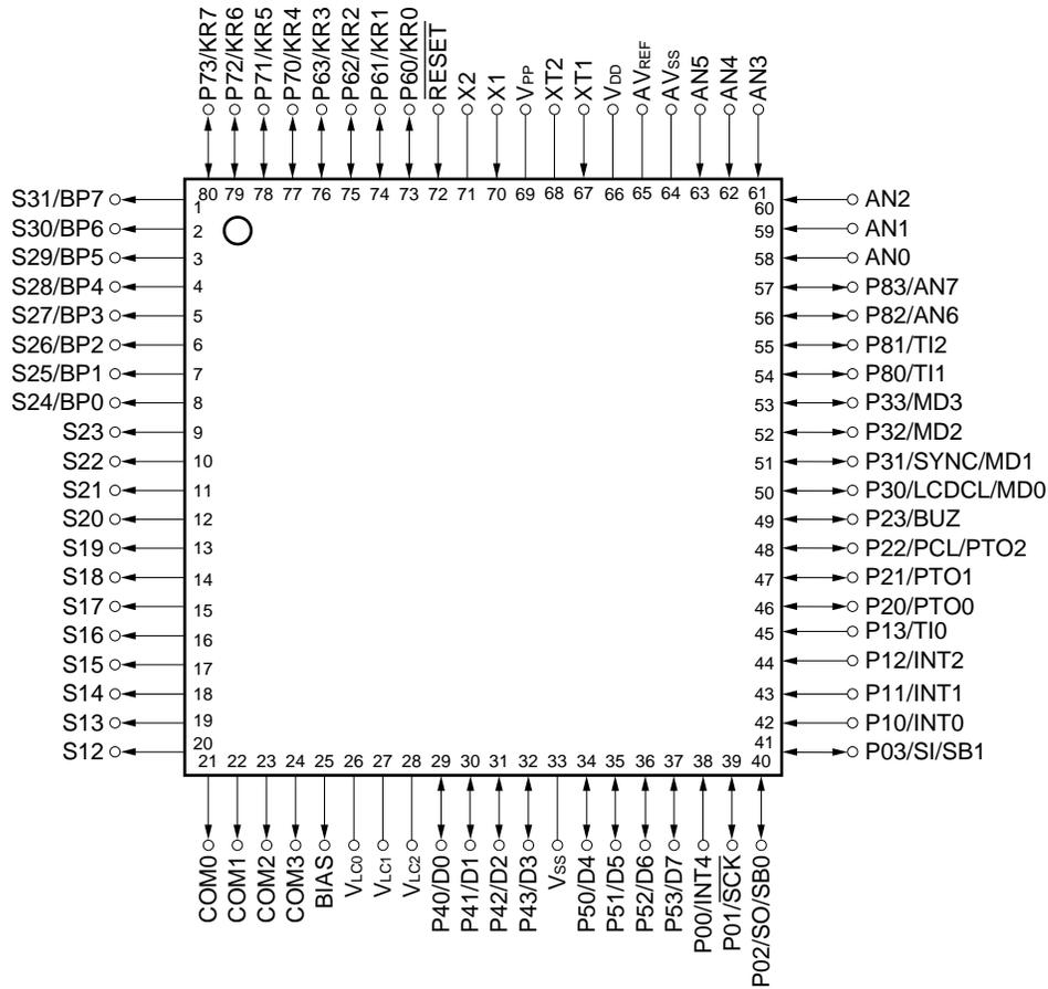
**Caution** Connect the V<sub>PP</sub> pin directly to V<sub>DD</sub>.
