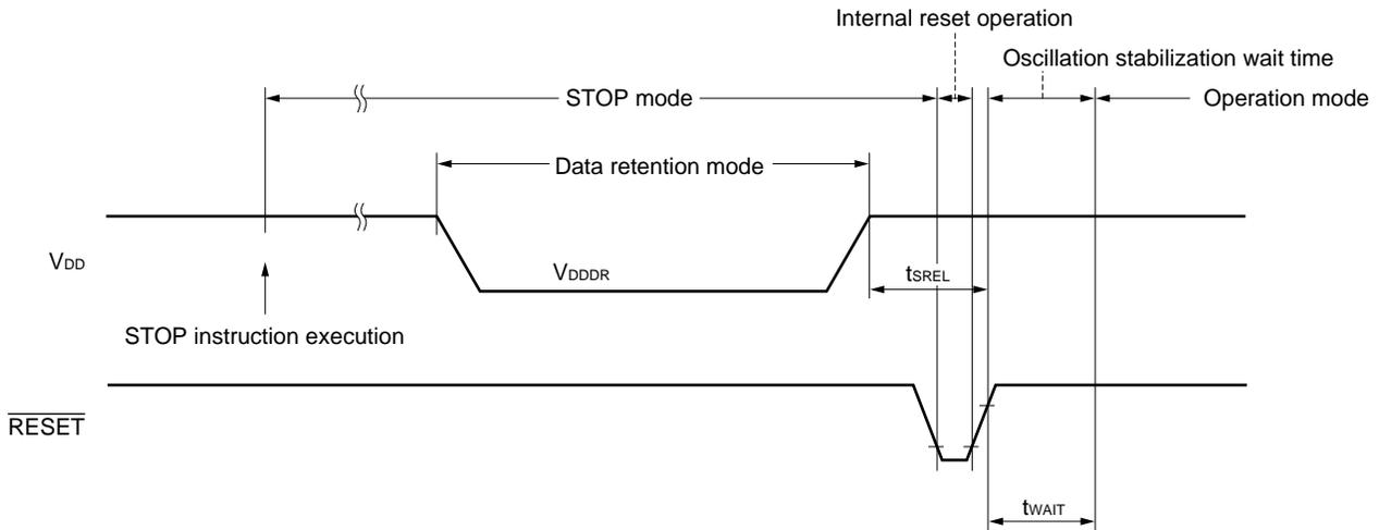
**Data retention timing (standby release signal: when STOP mode released by interrupt signal)**
