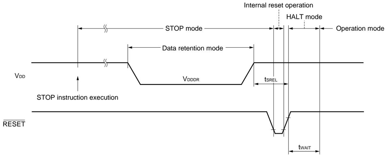
Data retention timing (standby release signal: when STOP mode released by interrupt signal)
