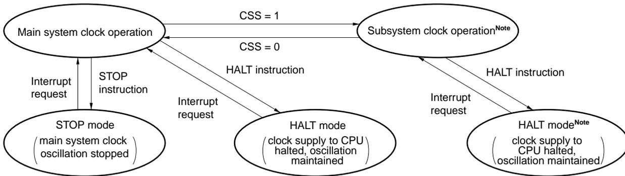
**Note** The current consumption can be reduced by stopping the main system clock. When the CPU is operating on the subsystem clock, set bit 7 (MCC) of the processor clock control register (PCC) to stop the main system clock. The STOP instruction cannot be used.
