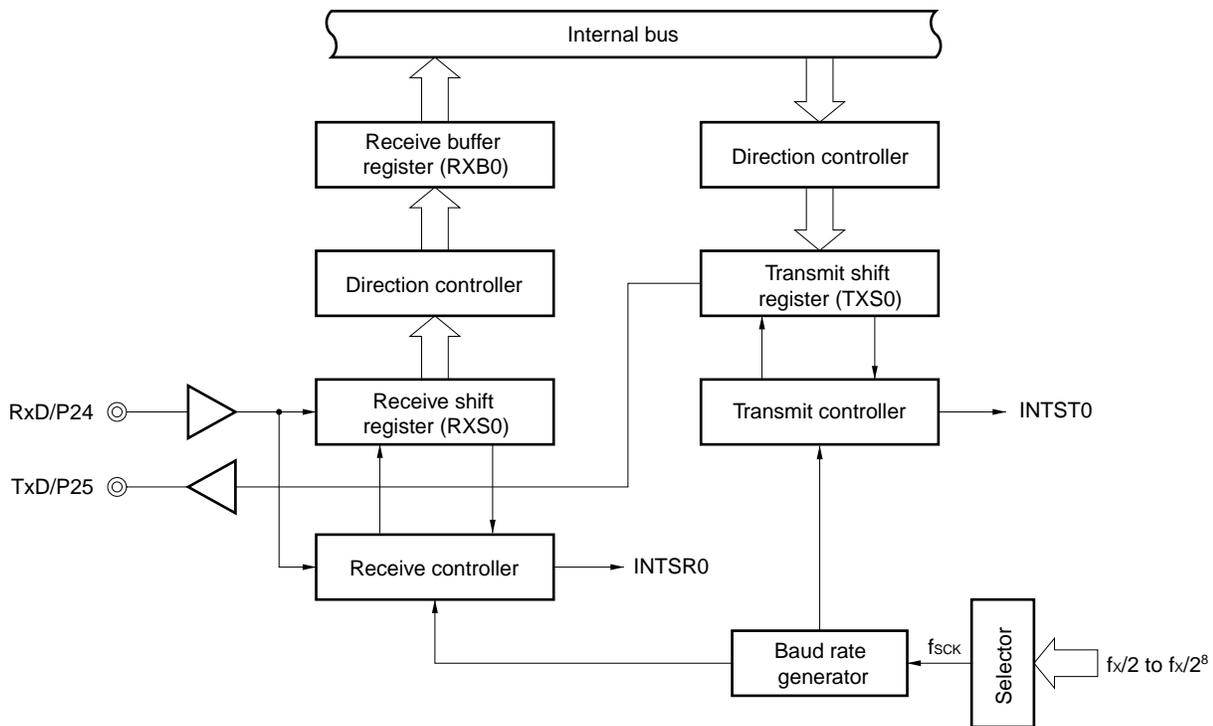
Figure 5-10. Block Diagram of Serial Interface SIO3
