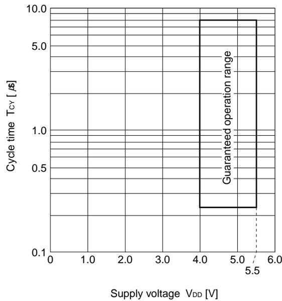
(2) Serial interface (T<sub>A</sub> = -40 to +85°C, V<sub>DD</sub> = 4.0 to 5.5 V)
