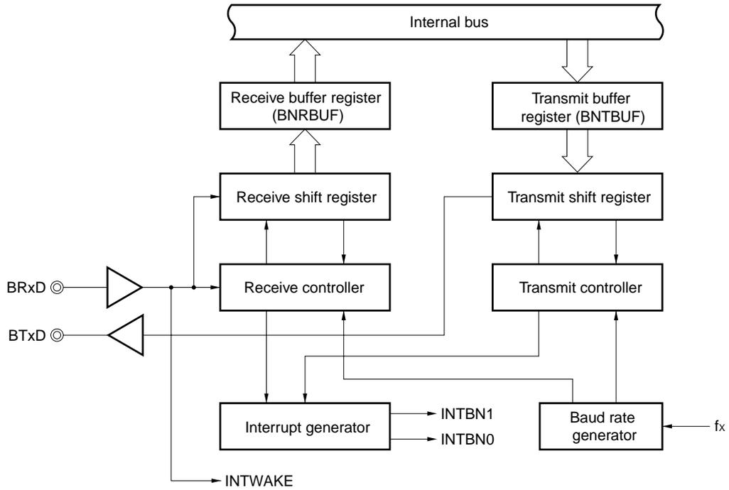
Figure 5-9. Block Diagram of Serial Interface UART
