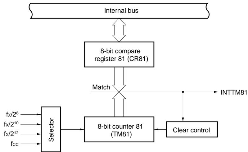
Figure 5-6. Block Diagram of Watchdog Timer
