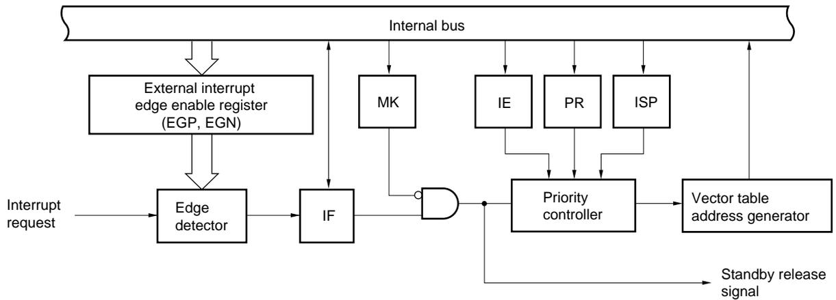
Figure 6-1. Basic Configuration of Interrupt Function (2/2)
