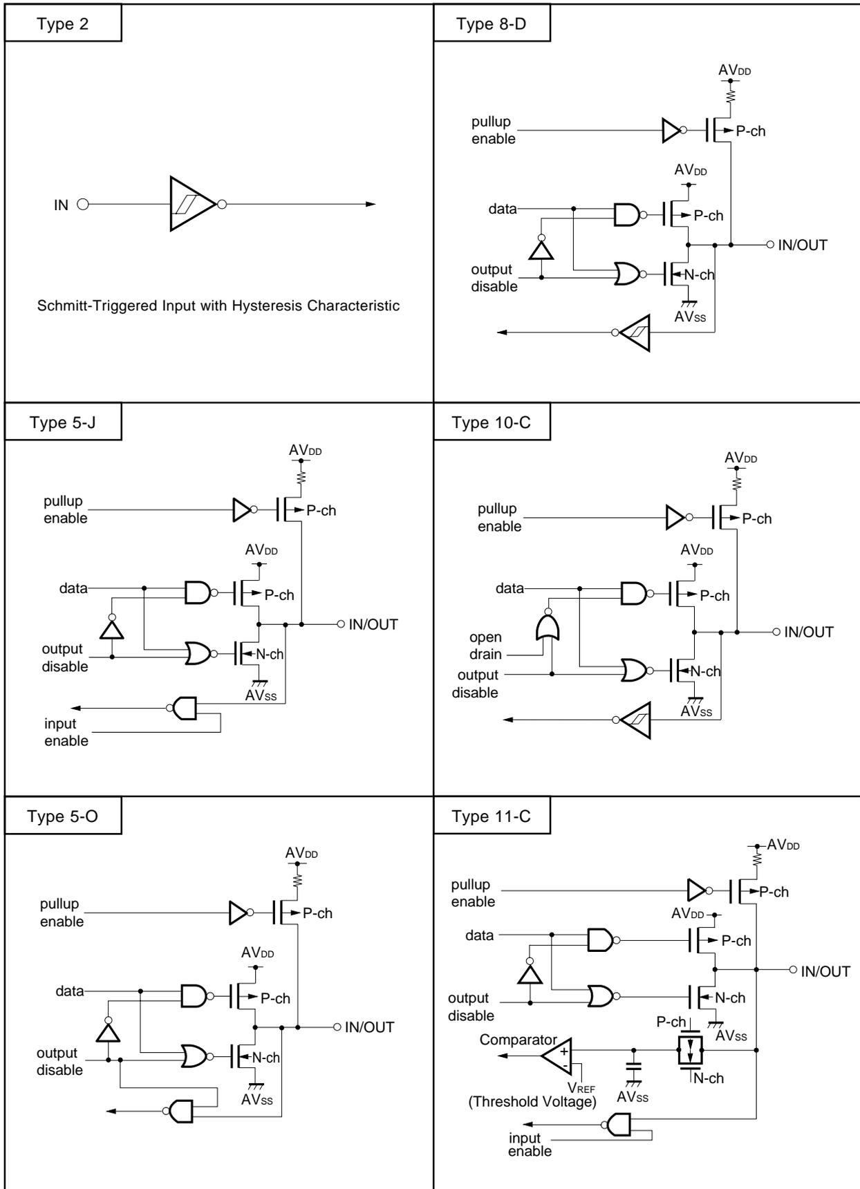
Figure 2-1. Pin Input/Output Circuits (2/2)
