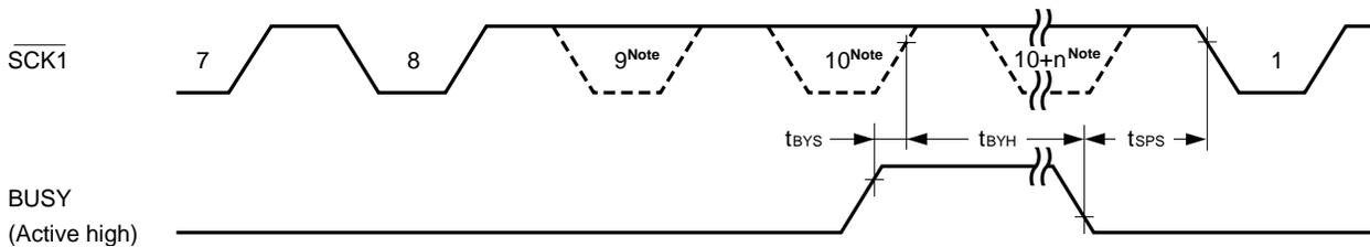
**Note** The signal is not actually low here, but is represented this way to show the timing.
