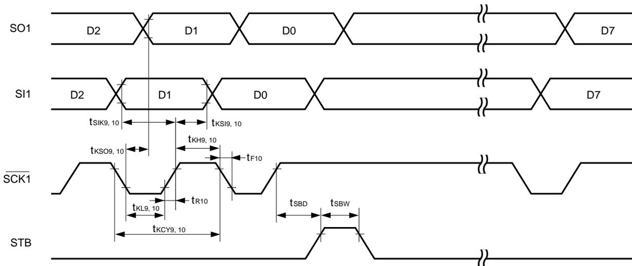
Automatic transmission/reception function 3-wire serial I/O mode (busy processing):
