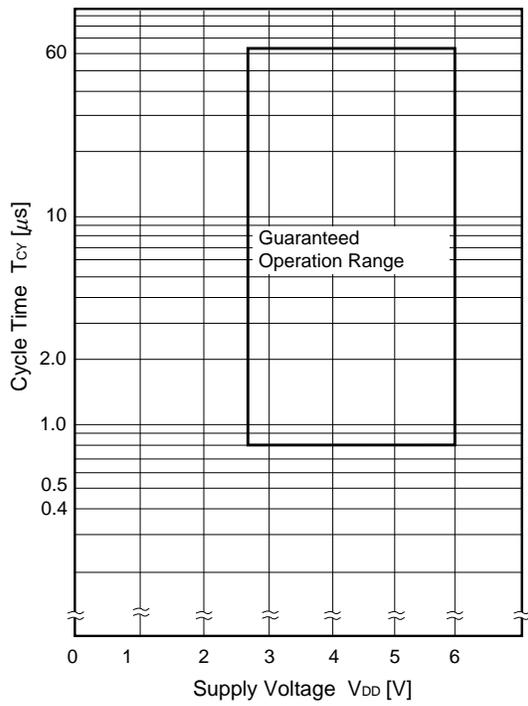
**T<sub>CY</sub> vs V<sub>DD</sub> (Main System Clock, f<sub>XX</sub> = f<sub>X</sub>)**
