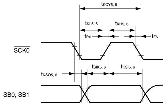
Automatic transmission/reception function 3-wire serial I/O mode:
