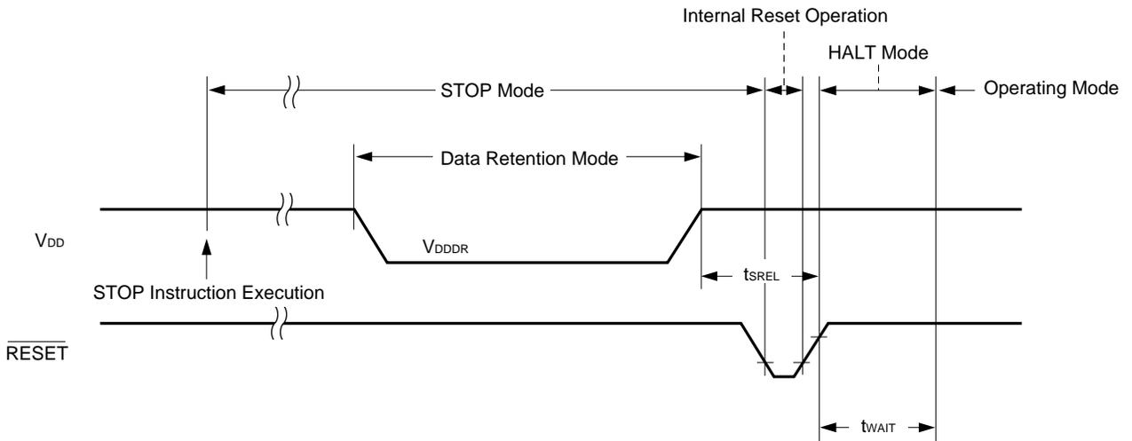
**Data Retention Timing (Standby release signal: STOP mode release by interrupt signal)**
