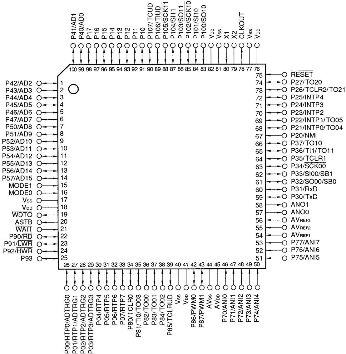
**Caution** Connect the MODE0 and MODE1 pins directly to the V<sub>SS</sub> pins.
