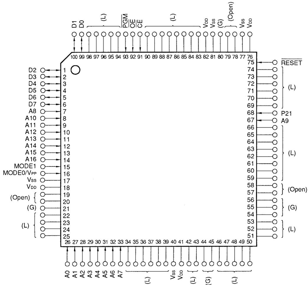
**Caution** Symbols in parentheses denote how the pins not used in the PROM programming mode should be treated.
