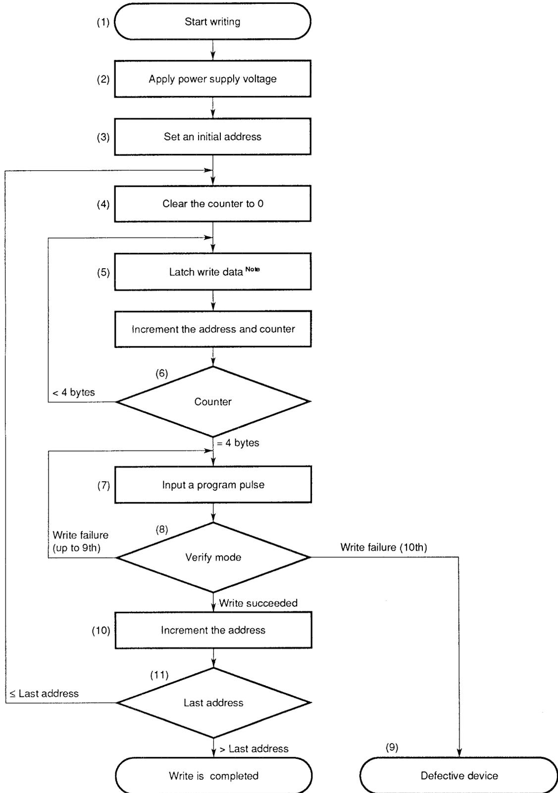
**Note** If write data does not fill a page, latch FFH for the rest of the page.
