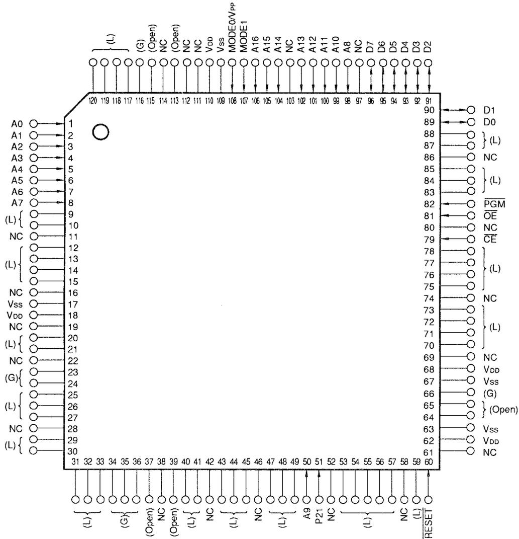
**Caution** Symbols in parentheses denote how the pins not used in the PROM programming mode should be treated.
