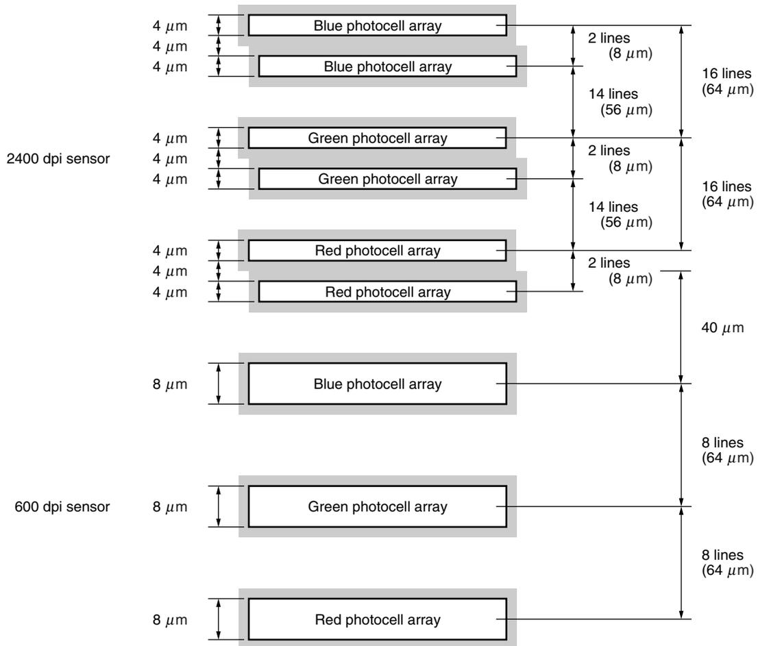
**PHOTOCELL ARRAY STRUCTURE DIAGRAM 2 (The Relation of the Photocell Array)**
