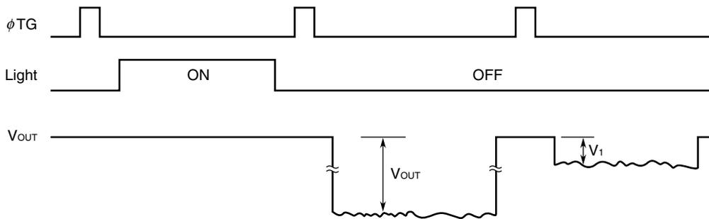
$$IL (\%) = \frac{V_1}{V_{OUT}} \times 100$$
