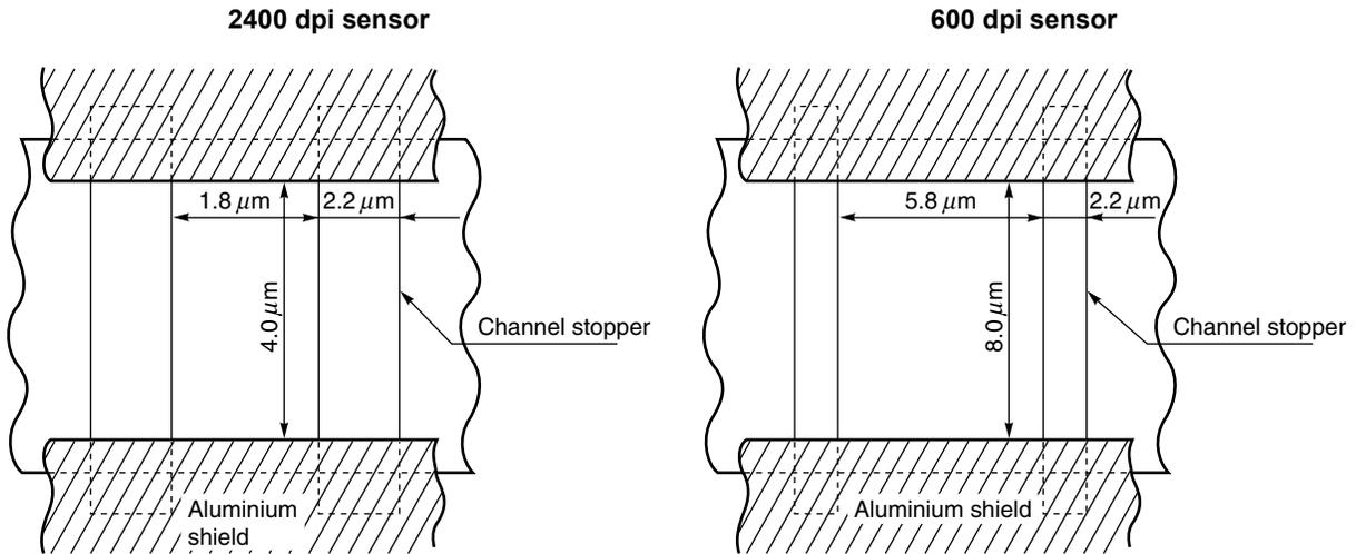
PHOTOCELL ARRAY STRUCTURE DIAGRAM 1 (Line Spacing)
