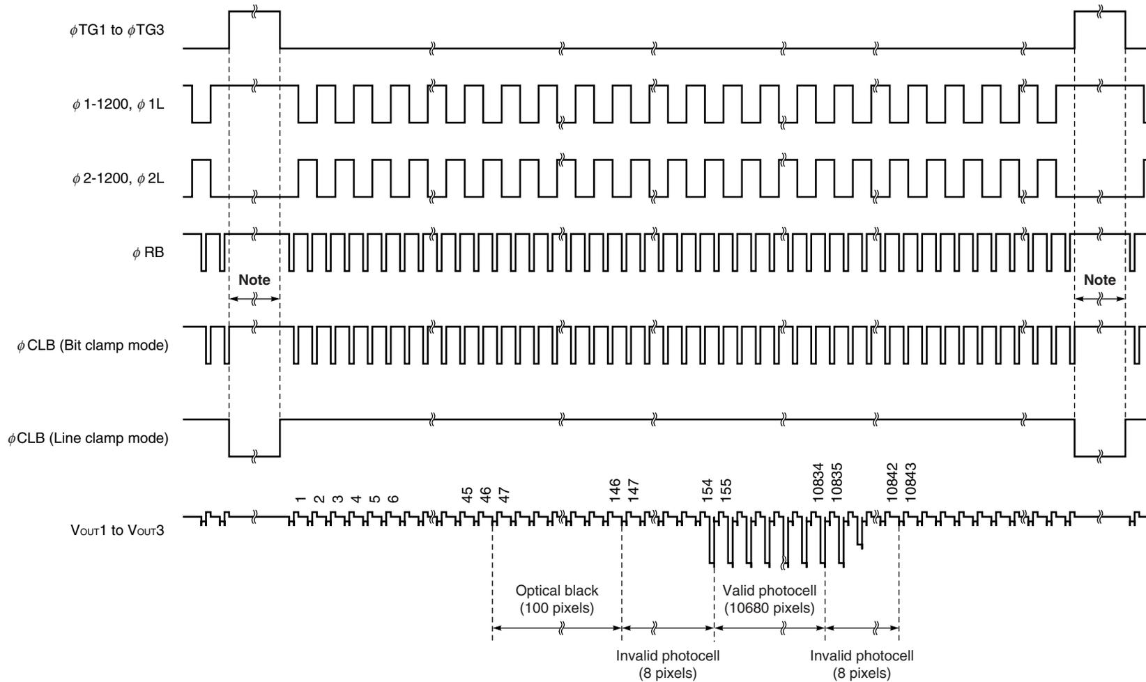
**Note** Set the  $\phi$  RB pulse and  $\phi$  CLB pulse (bit clamp mode) to high level during the  $\phi$  TG1 to  $\phi$  TG3 pulse.
