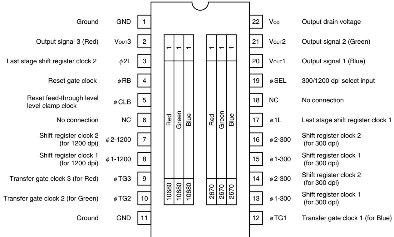
**Caution** Connect the No connection pins (NC) to GND.
