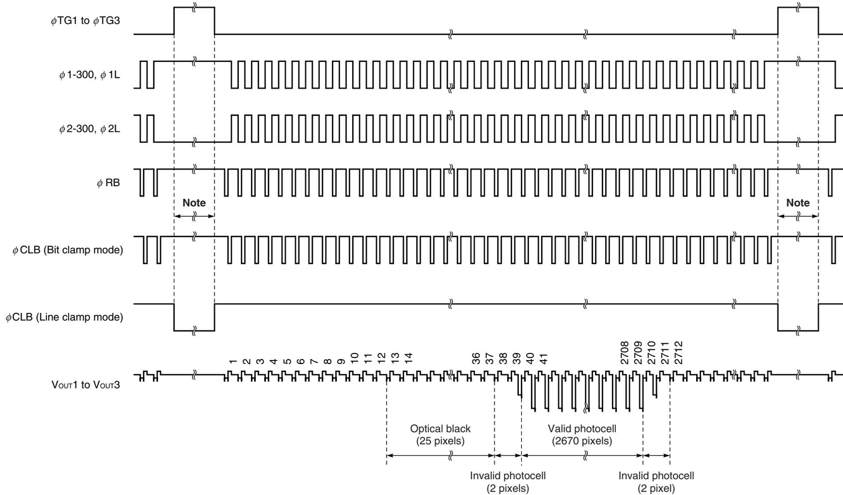
**Note** Set the  $\phi RB$  pulse and  $\phi CLB$  pulse (bit clamp mode) to high level during the  $\phi TG1$  to  $\phi TG3$  pulse.
