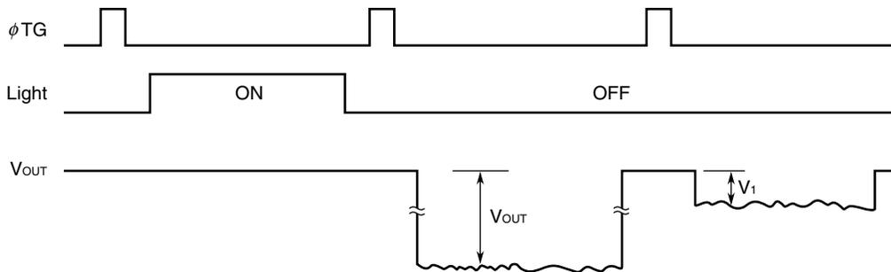
$$\text{IL (\%)} = \frac{V_1}{V_{\text{OUT}}} \times 100$$
