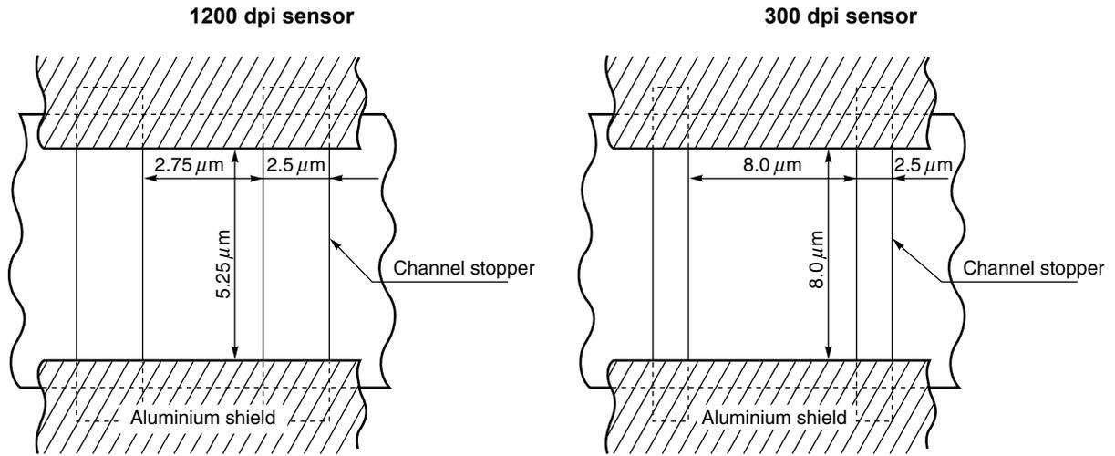
PHOTOCELL ARRAY STRUCTURE DIAGRAM 1 (Line Spacing)
