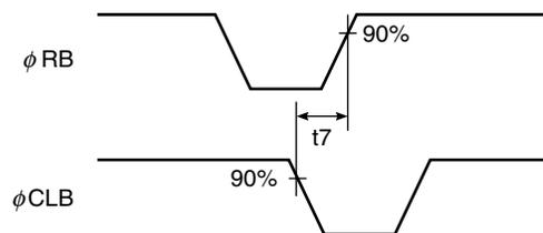
**Remark** Inverse pulse of the  $\phi TG1$  to  $\phi TG3$  can be used as  $\phi CLB$ .
