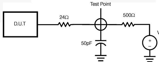
Figure 8. Load for Enable and Disable Times
