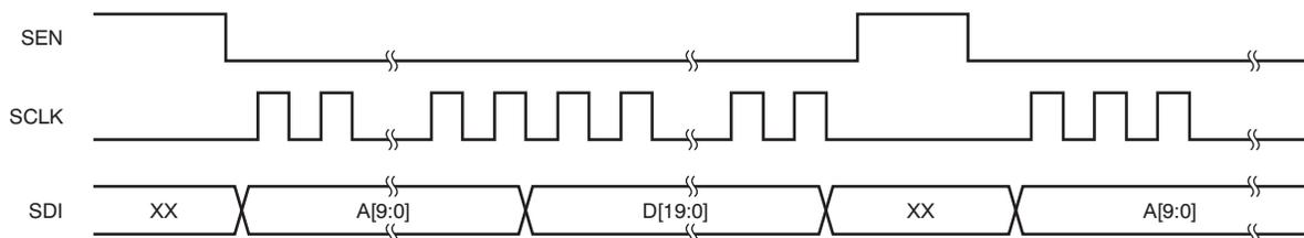
Figure 22. SPI Signal Flow of Write Mode
