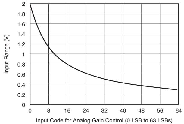
Figure 13. Input Range vs Analog Gain Setting Code
