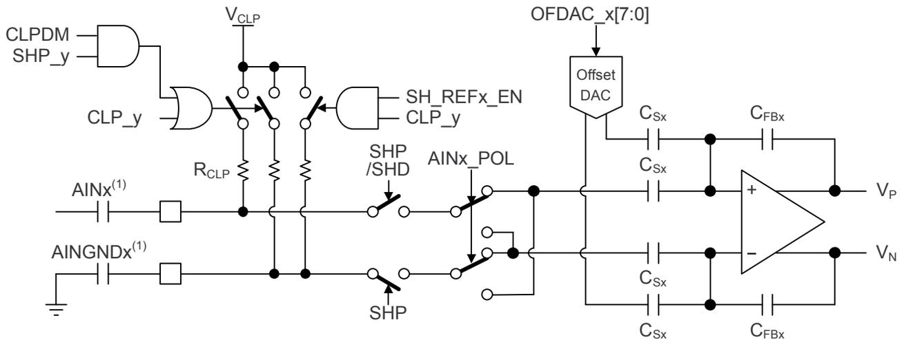
Figure 4. CDS Mode Input Circuit for CCD Signal
