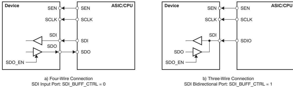
**Figure 23. SPI Connection Between AFE and System**
