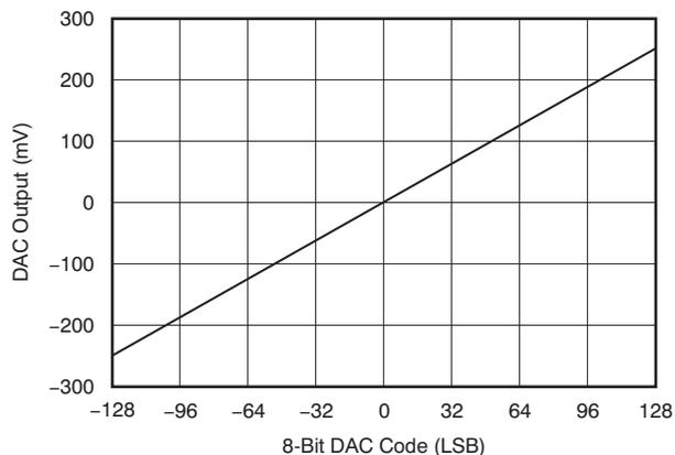
**Figure 15. Offset DAC Setting Code vs Output Voltage**
