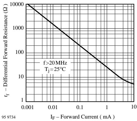
Figure 2. Differential Forward Resistance vs. Forward Current
