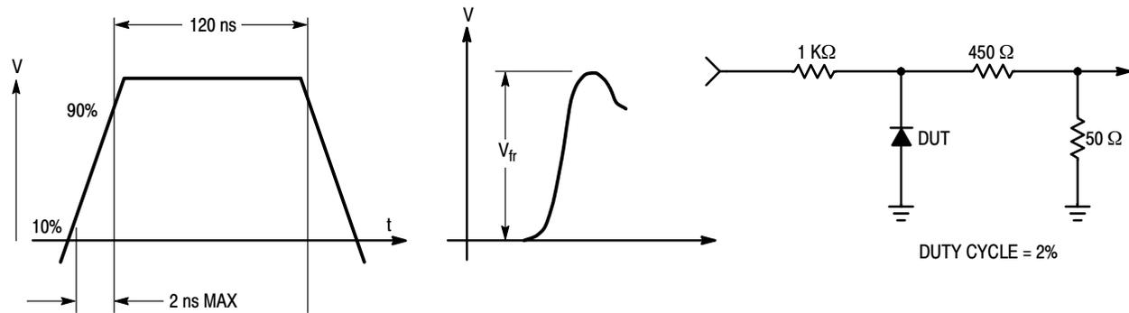
Figure 3. Forward Recovery Voltage Equivalent Test Circuit
