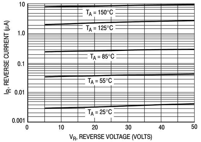
**Figure 5. Leakage Current**
