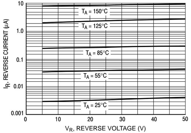
**Figure 3. Leakage Current**
