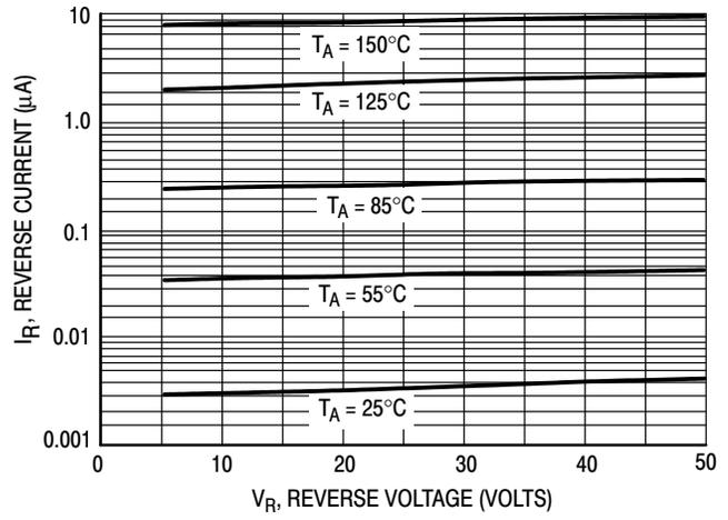
Figure 5. Leakage Current
