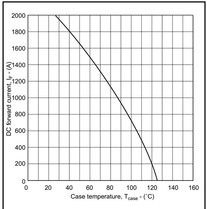
Fig. 6 DC current rating vs case temperature
