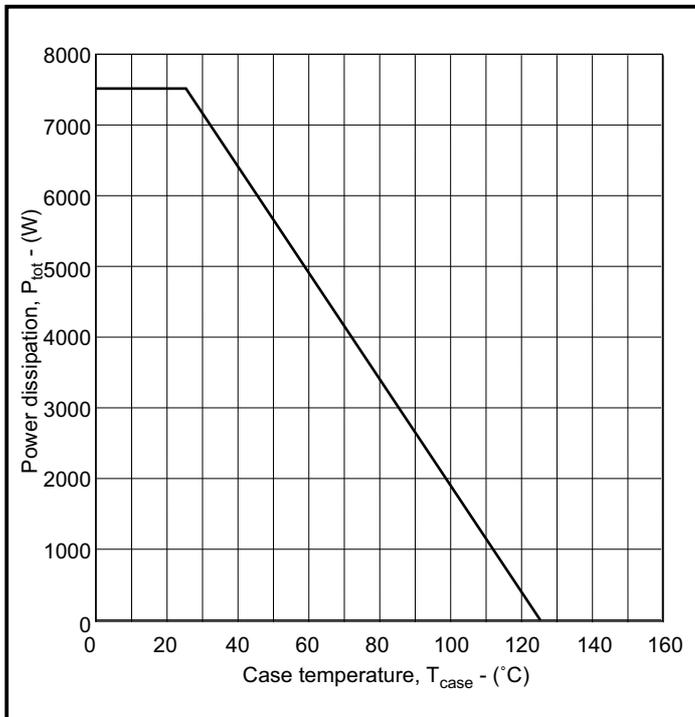
Fig. 5 Power dissipation
