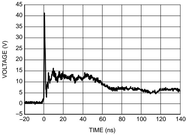
Figure 2. IEC61000-4-2 +8 kV Contact ESD Clamping Voltage
