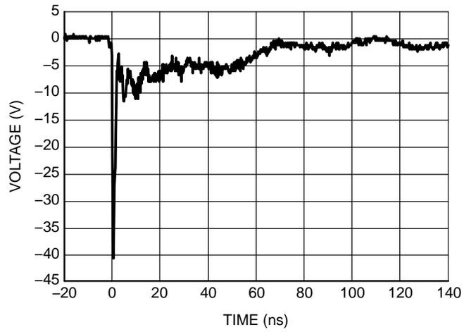
Figure 3. IEC61000-4-2 -8 kV Contact ESD Clamping Voltage
