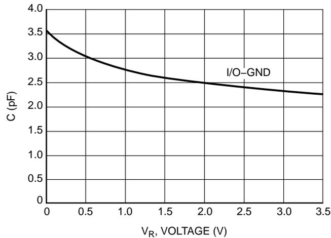
Figure 6. CV Characteristics
