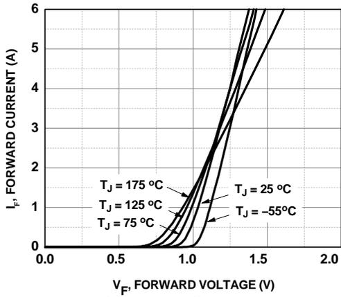
Figure 1. Forward Characteristics
