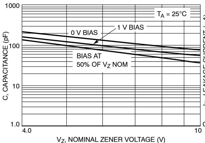
Figure 3. Typical Capacitance
