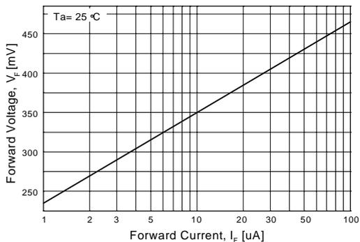
**Figure 3. Forward Voltage vs Forward Current**
