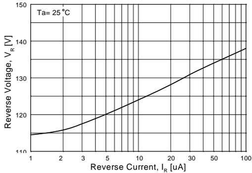
**Figure 1. Reverse Voltage vs Reverse Current**
