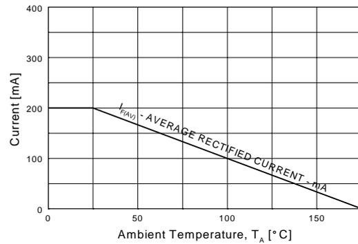
Figure 8. Average Rectified Current ( $I_{F(AV)}$ )
