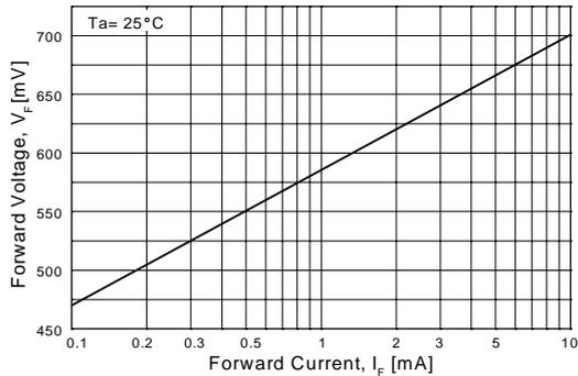
**Figure 4. Forward Voltage vs Forward Current**
