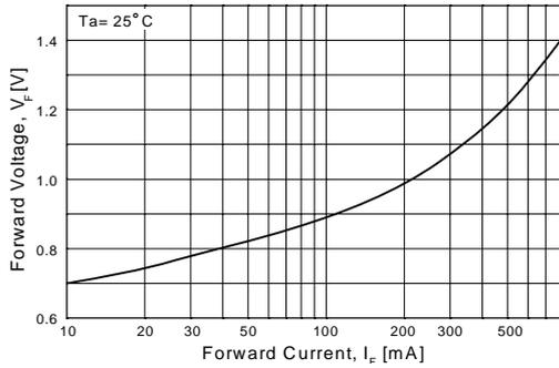
Figure 5. Forward Voltage vs Forward Current
