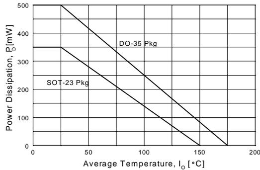
Figure 9. Power Derating Curve
