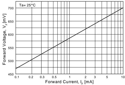
Figure 4. Forward Voltage vs Forward Current
