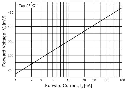
Figure 3. Forward Voltage vs Forward Current
