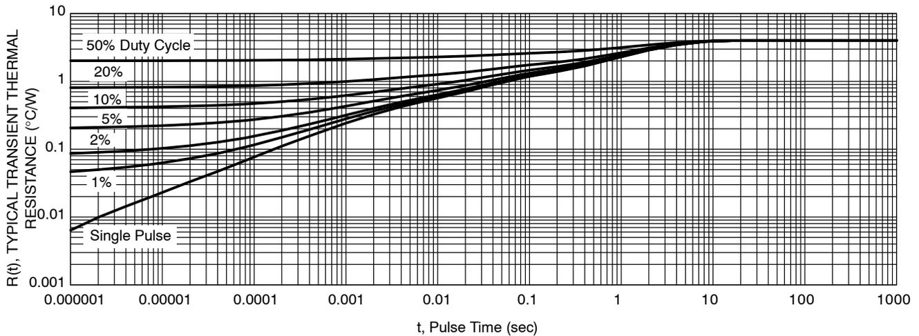
Figure 8. Typical Transient Thermal Response, Junction-to-Case for NTSJ30U100CTG
