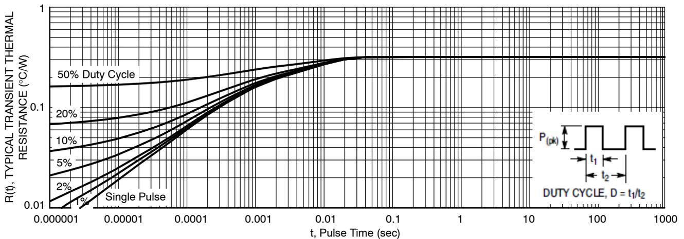
Figure 9. Typical Transient Thermal Response, Junction-to-Case for NTSB30U100CTG
