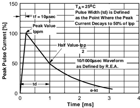
Figure 3. Pulse Waveform
