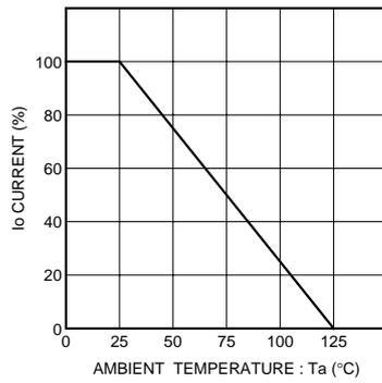
Fig. 5 Derating curve (mounting on glass epoxy PCBs)
