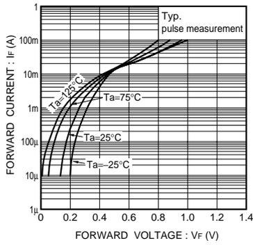
Fig. 1 Forward characteristics
