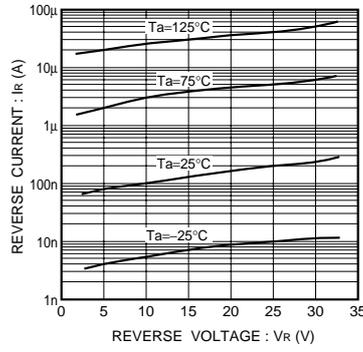
Fig. 2 Reverse characteristics
