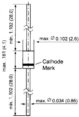
Dimensions are in inches and (millimeters)
