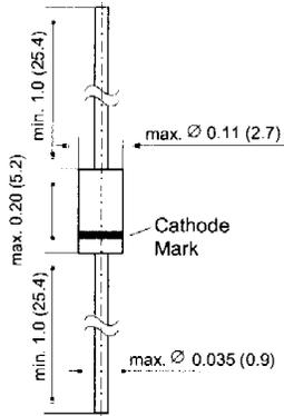
Dimensions are in inches and (millimeters)
