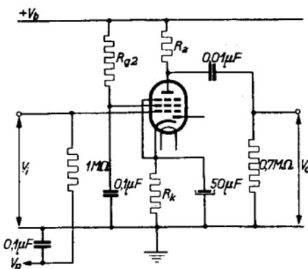
This valve can be used without special precautions against microphonic effect in circuits in which the input voltage  $V_i \geq 10$  mV for an output of 50 mW of the output valve ( $R_g = 1$  M $\Omega$ )
