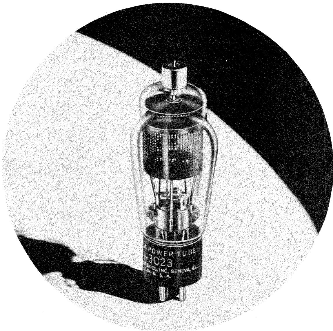
NATIONAL POWER TUBE NL-3C23 is a quick heating thyratron designed especially for industrial grid controlled rectifier applications. It is gas and mercury filled for quick starting and constancy of characteristics within wide temperature limits.
