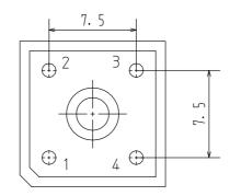
Dimensions with no tolerance specified  $\pm 1.0$
