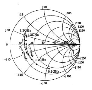
$S12e: V_{CE} = -10V \\ f = 100MHz, 200 \ \ \mbox{to} \ 1200MHz \, (200MHz \, step)$
