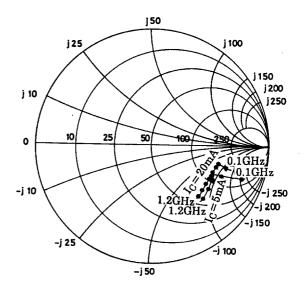
S Parameter (Common emitter)  $V_{CE} = -10V, I_C = -5mA, Zo = 50\Omega$
