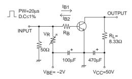
$I_C$ =10 $I_{B1}$ = -10 $I_{B2}$ =6A For PNP, the polarity is reversed.
