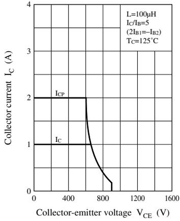
Safe operation area (Reverse bias) measurement circuit
