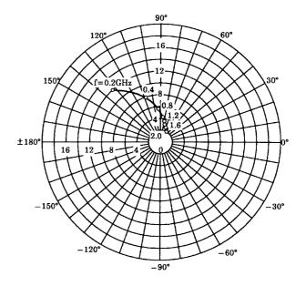
$\begin{array}{l} S_{12e} \\ V_{CE} = 10V \\ I_{C} = 5 mA \\ Ta = 25 ^{\circ}C \end{array}$
