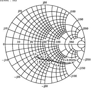
$\begin{array}{l} S_{11e} \\ V_{CE} = 10V \\ I_{C} = 20 mA \\ Ta = 25 ^{\circ}C \\ (Unit: \Omega) \end{array}$
