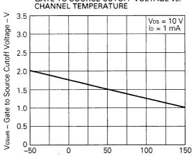
T<sub>ch</sub> – Channel Temperature – °C
