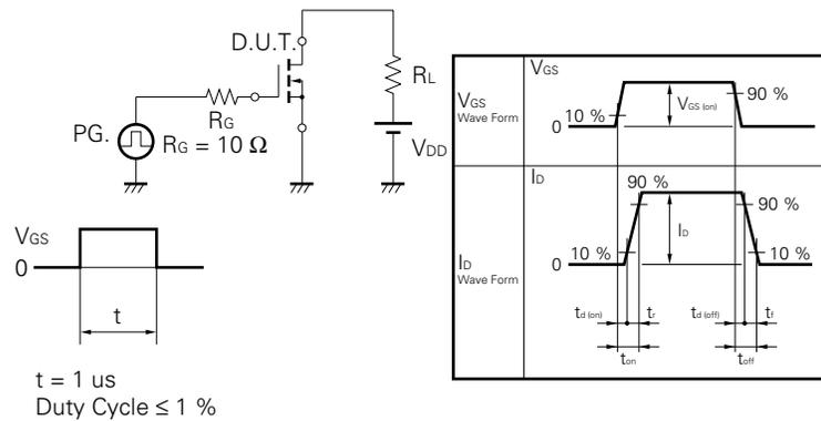
**Test Circuit 3 Gate Charge**
