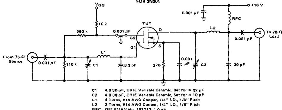
FIGURE 2 - 200-MHz-to-45-MHz TEST CIRCUIT SCHEMATIC FOR 3N202
