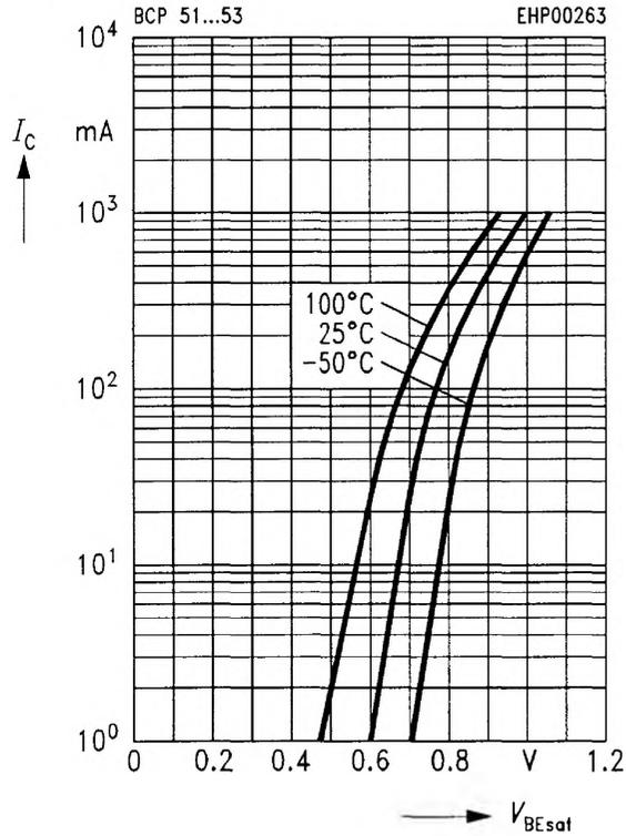
**Collector-emitter saturation voltage**
